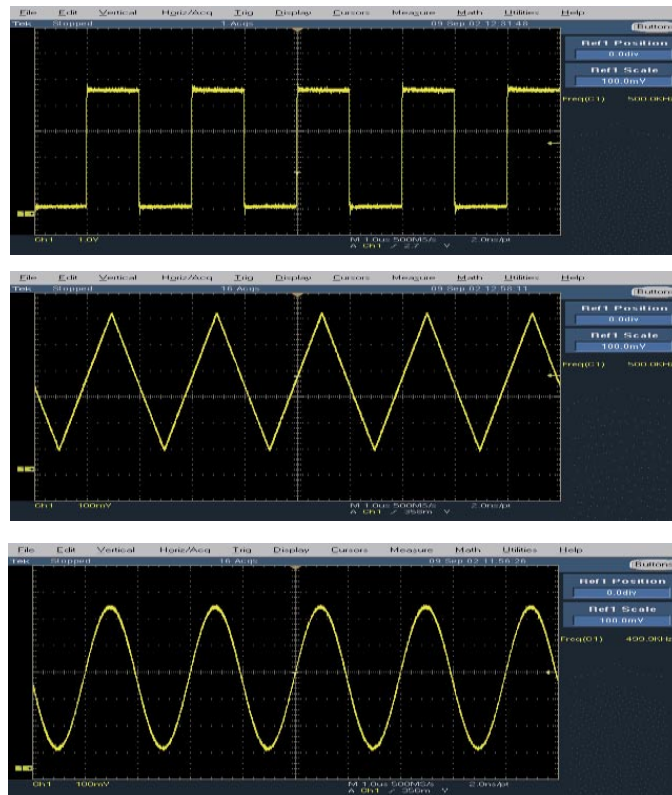
Figure 2. Square-, triangular-, and sinusoidal outputs from a DDS.
