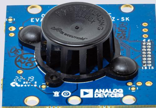
Figure 1. Evaluation board attached to chamber, top view.
