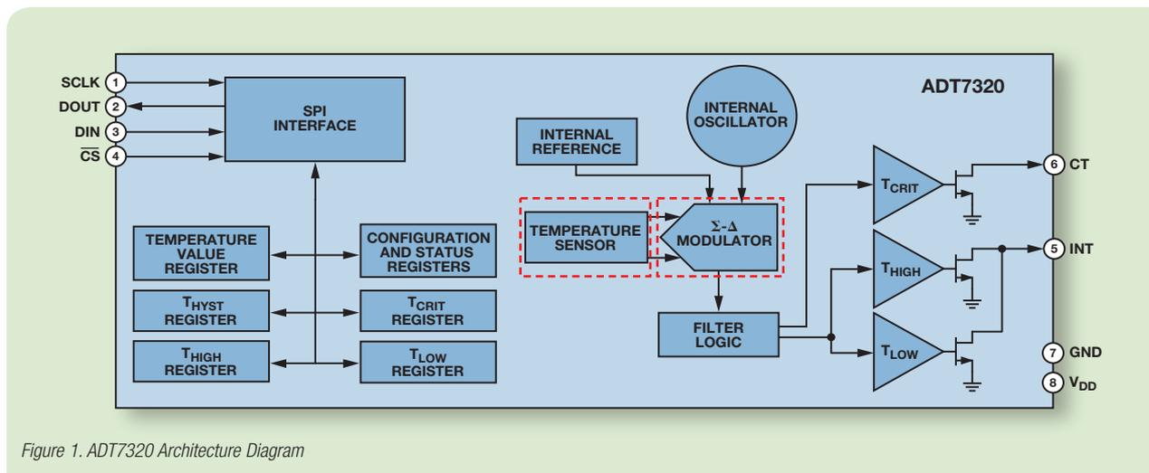
Figure 1. ADT7320 Architecture Diagram
