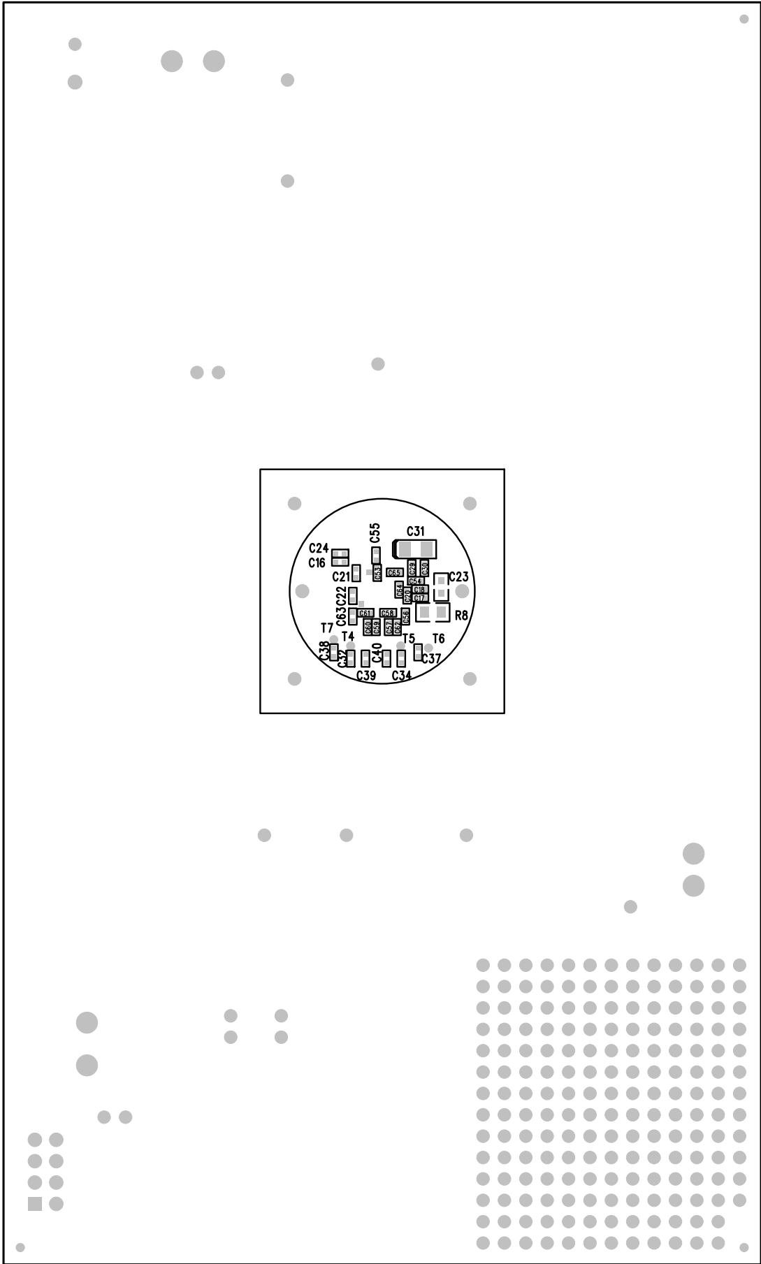
EVAL-ADuCM310EBZ (Rev C) Top Side View Bottom Side Silkscreen
