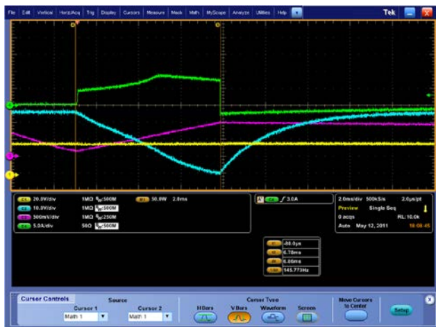
Figure 13. TIMER During a Fault; Channel 1 = VIN (Yellow); Channel 2 = V DS (Blue); Channel 3 = TIMER (Pink); Channel 4 = System Current (Green)
