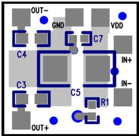
Figure 5. Bottom Layer with Bottom Silkscreen (Mirror Image)
