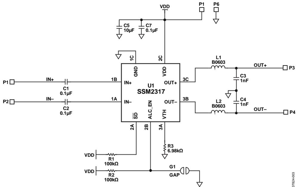
Figure 3. Schematic of the SSM2317-MINI Evaluation Board
