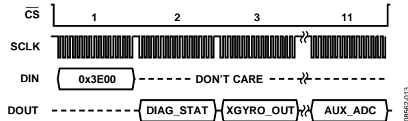
Figure 13. Burst Read Sequence
