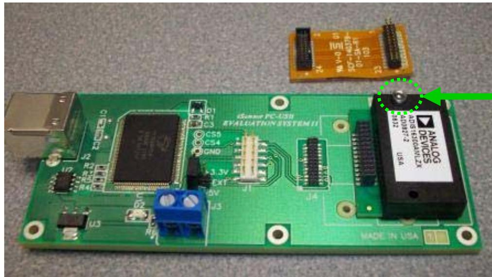
Move the ADIS16300AMLZ over the ADISUSBZ's holes for the ADIS1635x products and use (1) 2x10mm machine screw to attach the product. A 2mm washer may help with attachment strength as well.
