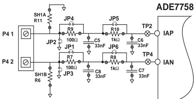
Figure 1 — Current Channel on the ADE7758 evaluation board
