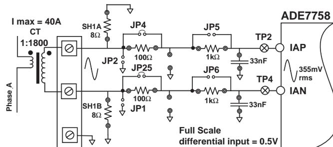
Figure 2 — CT connection to Current Channel
