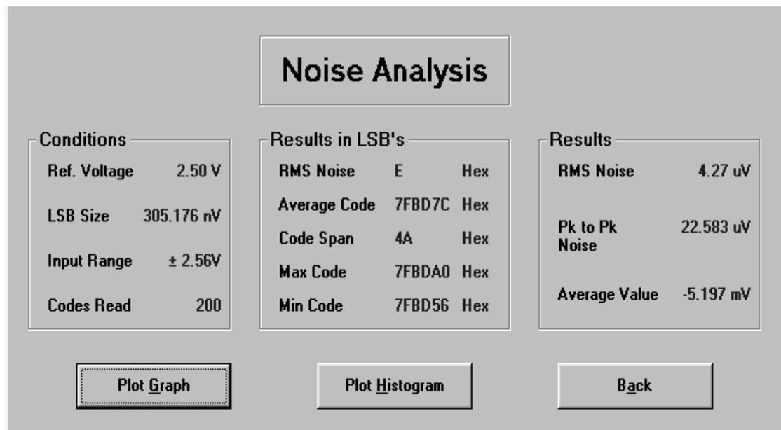
Fig. 6. The ADC Noise Analysis Screen
