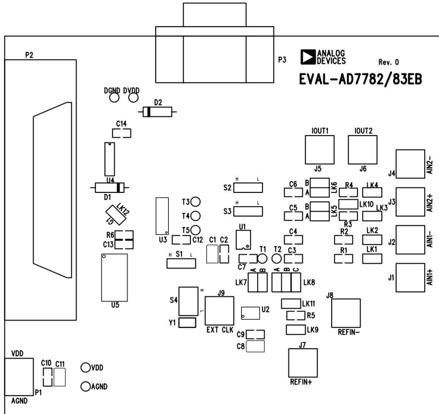
Fig. 22. The Evaluation Board Component Layout Diagram
