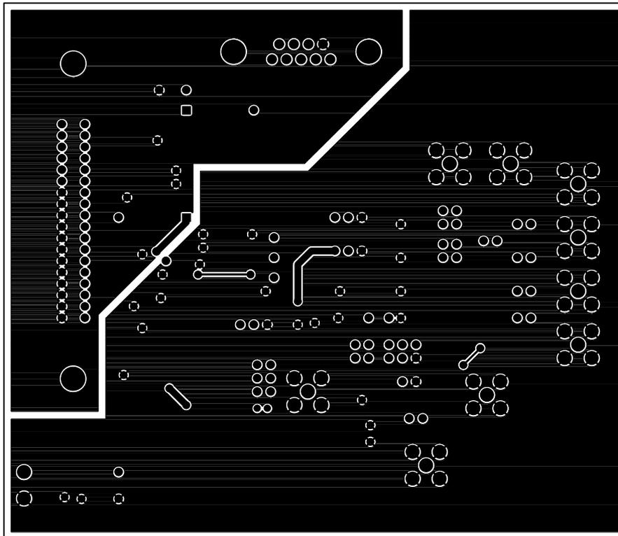
Fig. 23. The Evaluation Board SolderSide Artwork
