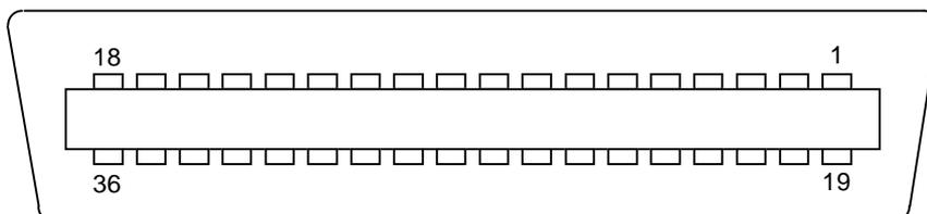
Fig. 3: 36-way Centronics (P2) Pin Configuration
