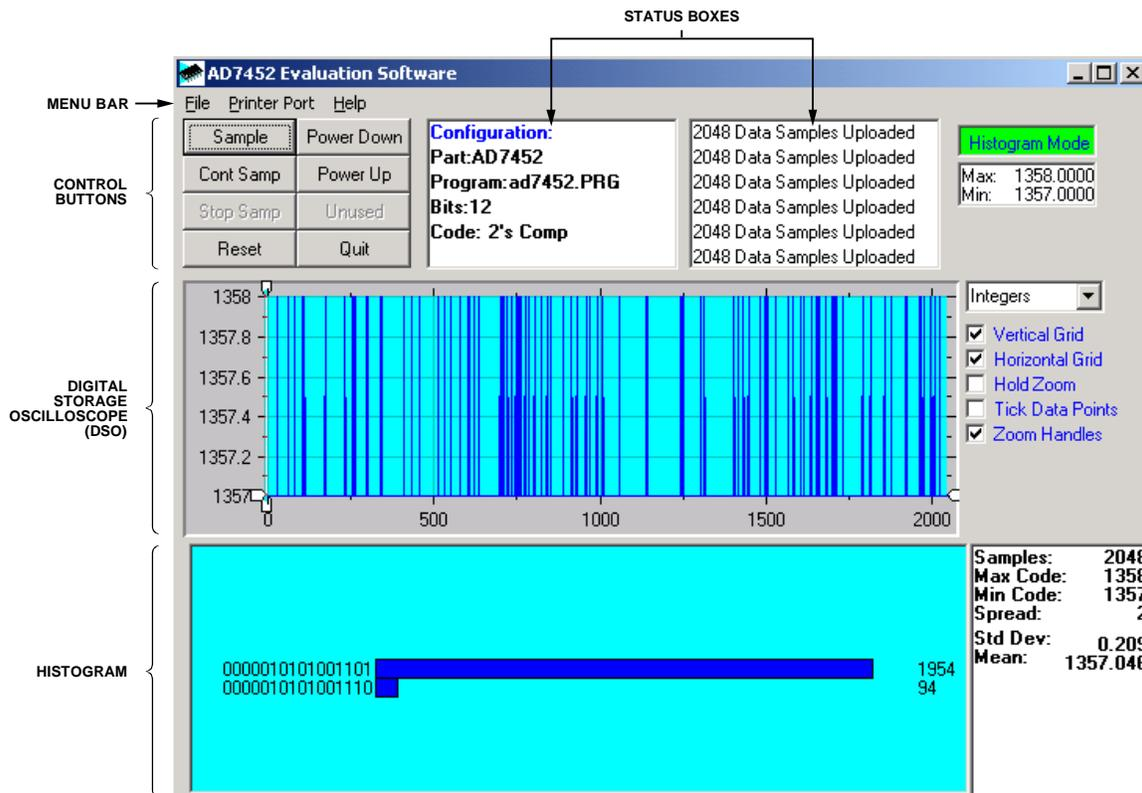
Figure 4. AD7452 Main Window–Histogram Mode
