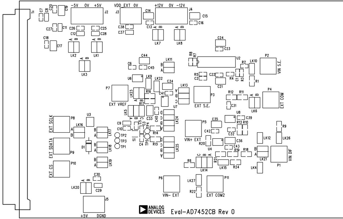
Figure 9. AD7452 Evaluation Board Component Placement Drawing
