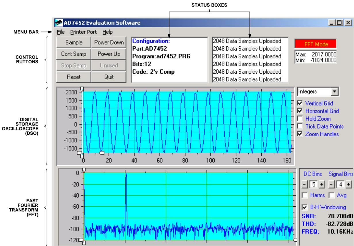
Figure 3. AD7452 Main Window—FFT Mode
