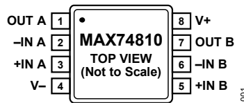
Figure 1. MAX74810 Pin Configuration
