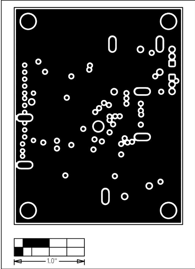
Figure 4. MAX17020 EV Kit PCB Layout—Layer 2 (PGND Plane)
