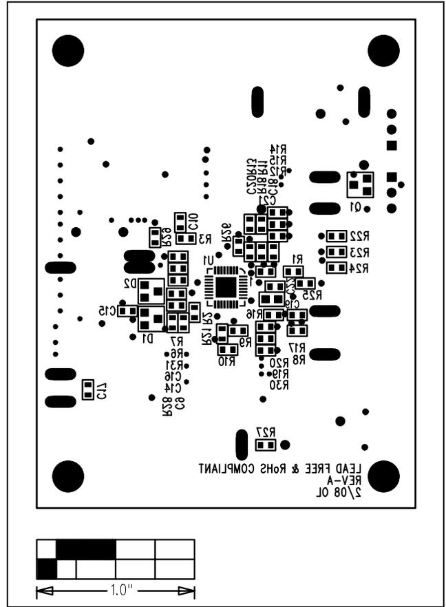
Figure 7. MAX17020 EV Kit Component Placement Guide—Solder Side
