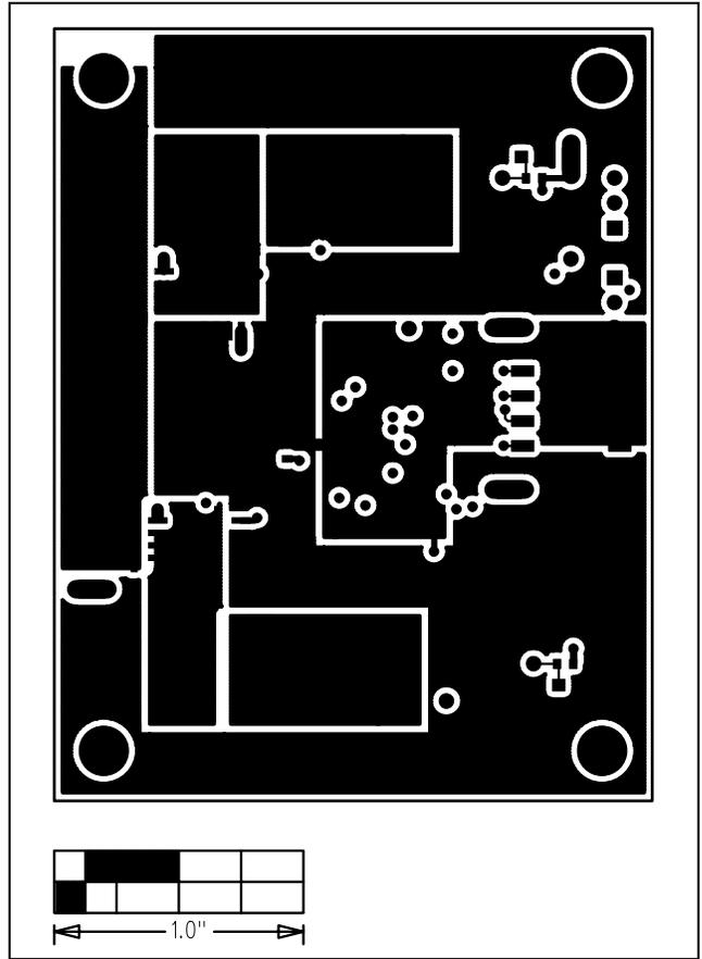
Figure 3. MAX17020 EV Kit PCB Layout—Component Side
