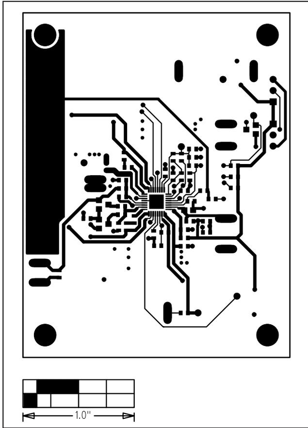
Figure 6. MAX17020 EV Kit PCB Layout—Solder Side
