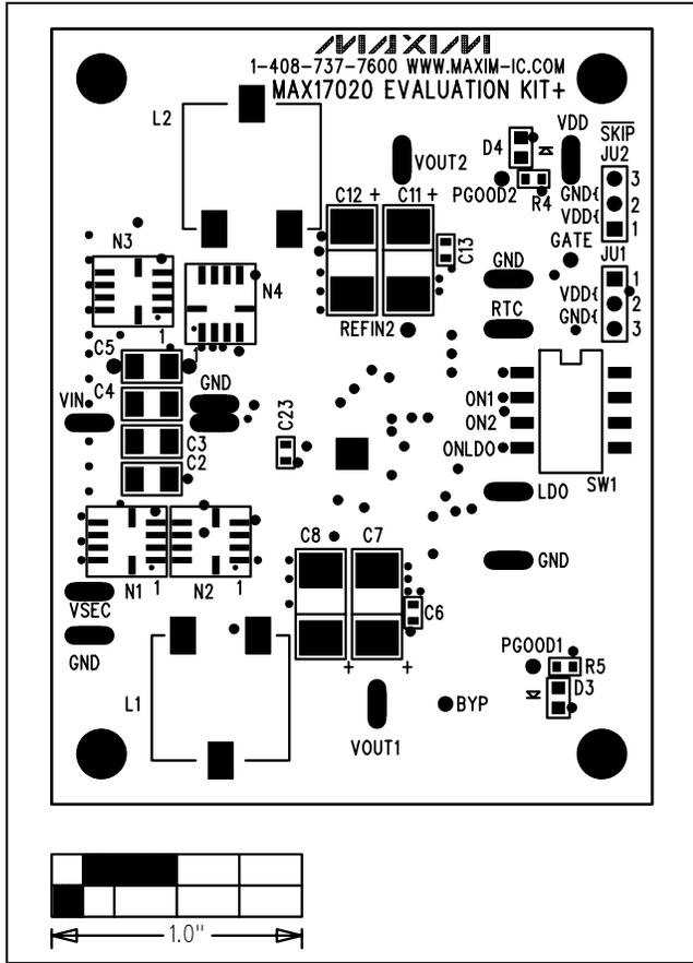
Figure 2. MAX17020 EV Kit Component Placement Guide—Component Side
