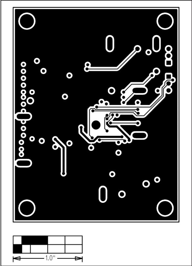
Figure 5. MAX17020 EV Kit PCB Layout—Layer 3 (PGND/Signal Layer)
