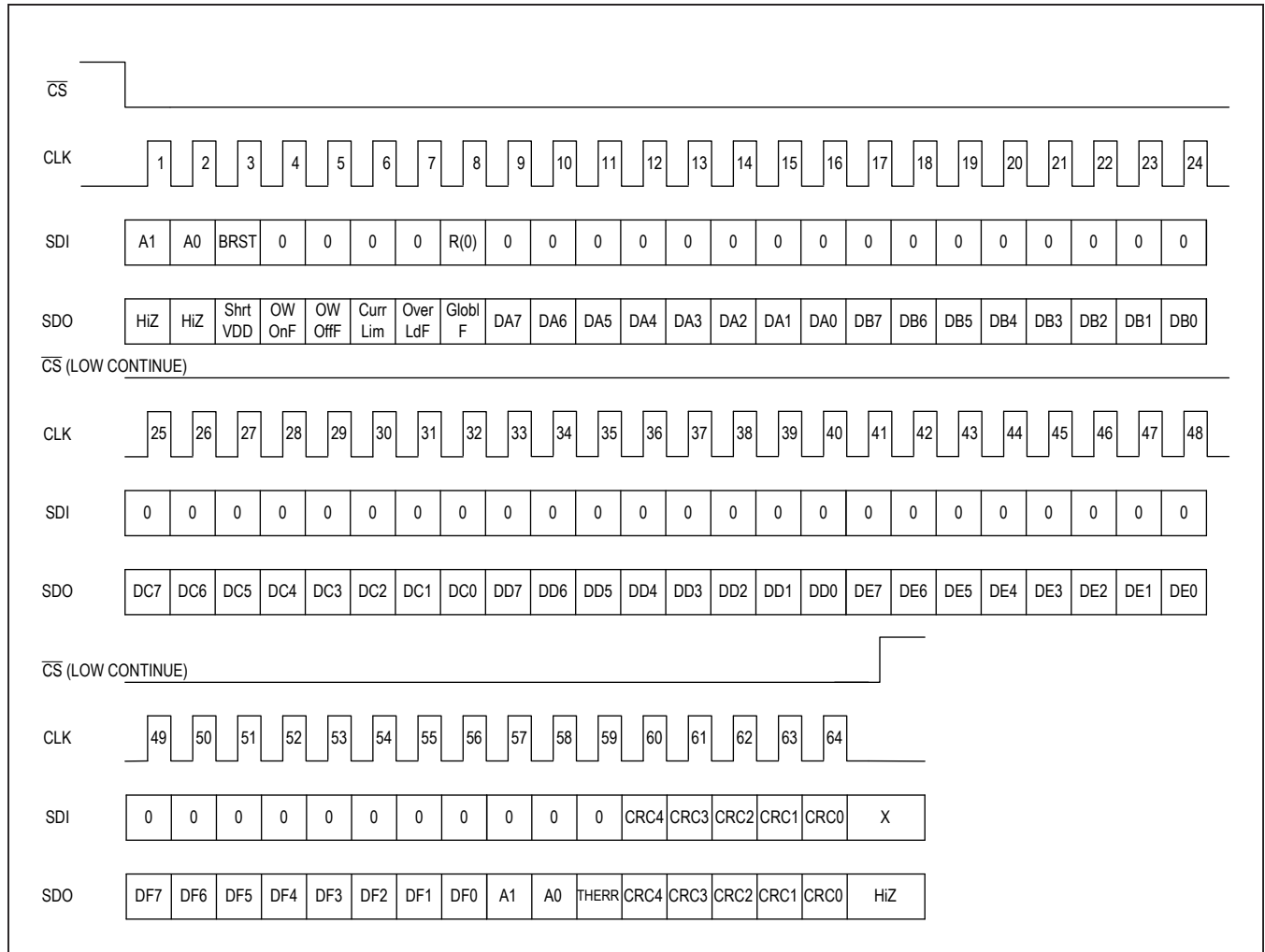
Figure 16. Addressed SPI Burst Read Command with CRC
