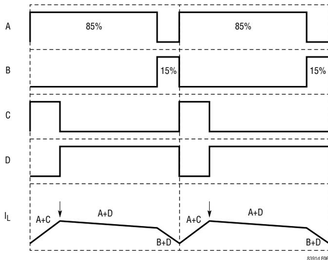
Figure 6. Peak-Boost in Buck-Boost Region ( $V_{IN} \lesssim V_{OUT}$ )
