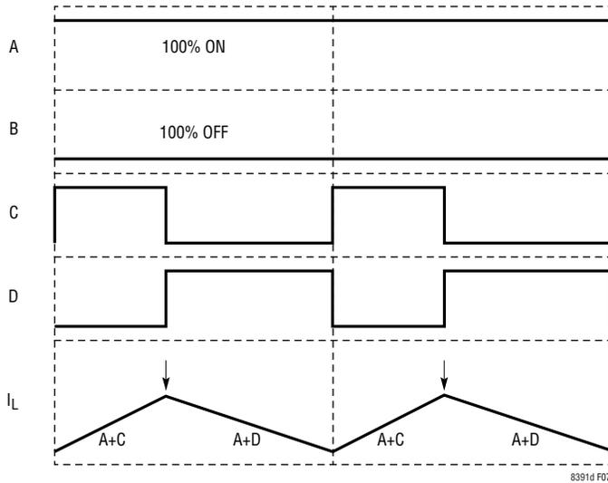
Figure 7. Peak-Boost in Boost Region ( $V_{IN} \ll V_{OUT}$ )
