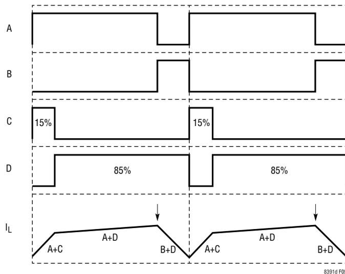
Figure 5. Peak-Buck in Buck-Boost Region ( $V_{IN} \sim V_{OUT}$ )
