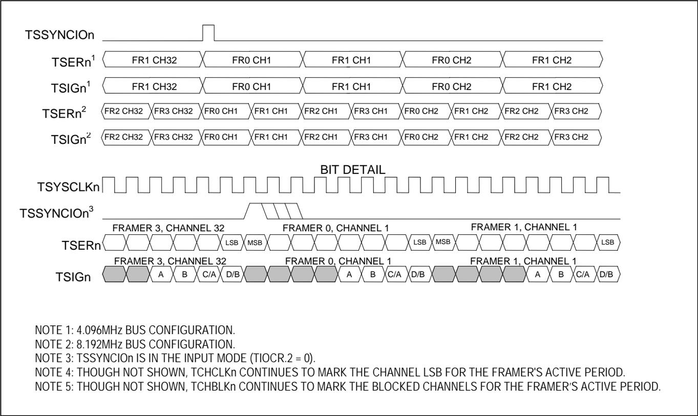
**Figure 11-15. T1 Transmit-Side Interleave Bus Operation—FRAME Mode**
