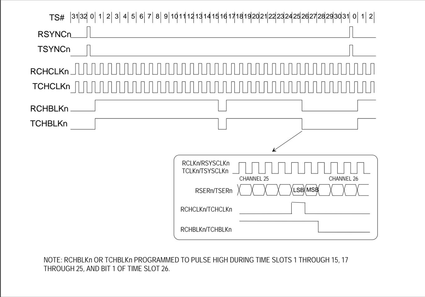
**Figure 11-31. E1 Transmit-Side TCHCLKn Gapped Mode During Channel 1**
