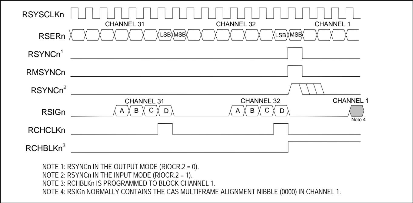
Figure 11-21. E1 Receive-Side Interleave Bus Operation—BYTE Mode
