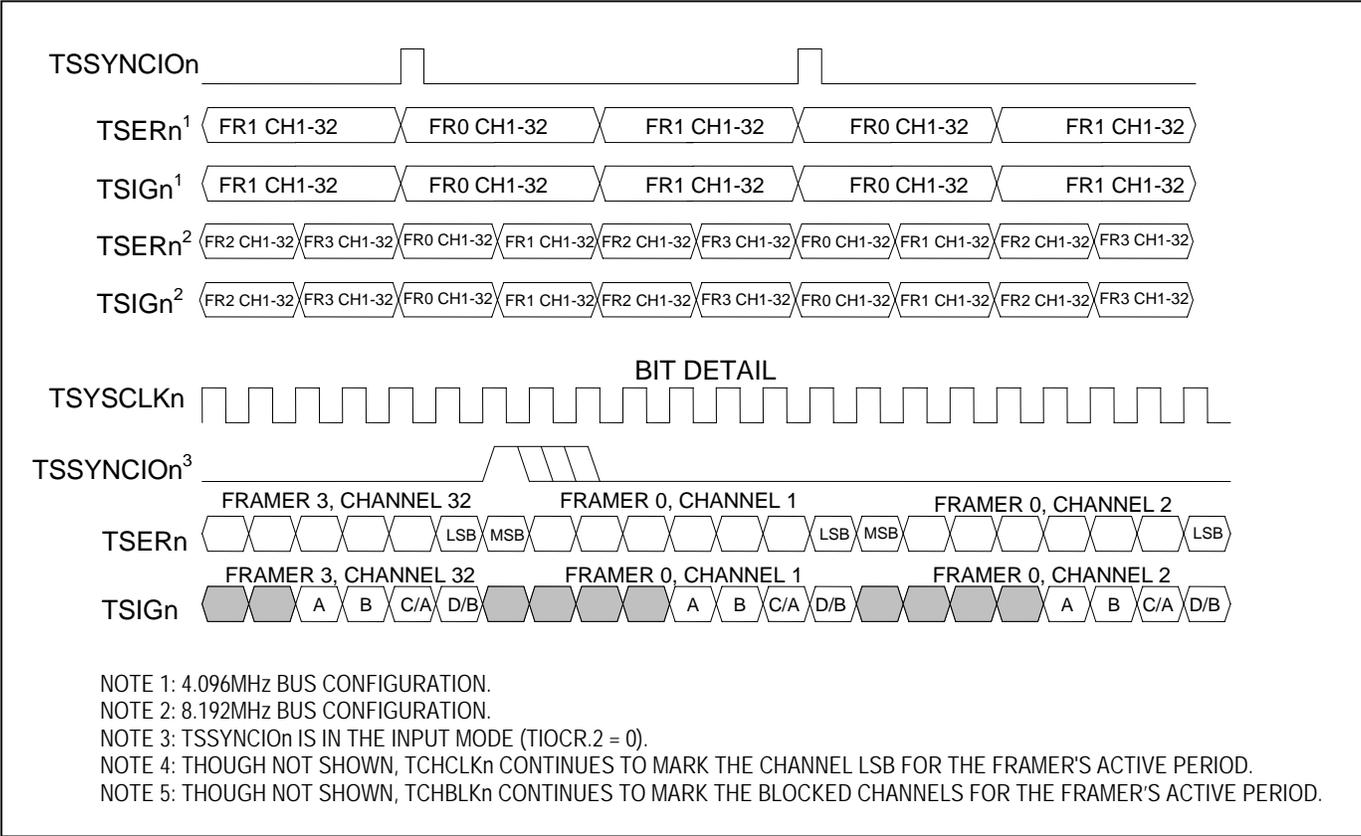
**Figure 11-16. T1 Transmit-Side TCHCLKn Gapped Mode During F-Bit**
