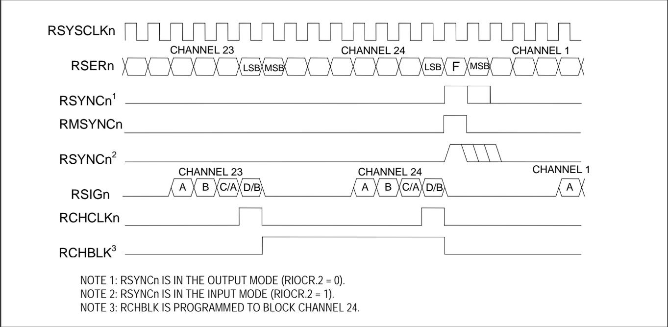
Figure 11-5. T1 Receive-Side 2.048MHz Boundary Timing (Elastic Store Enabled)
