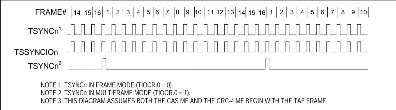
Figure 11-25. E1 Transmit-Side Boundary Timing (Elastic Store Disabled)
