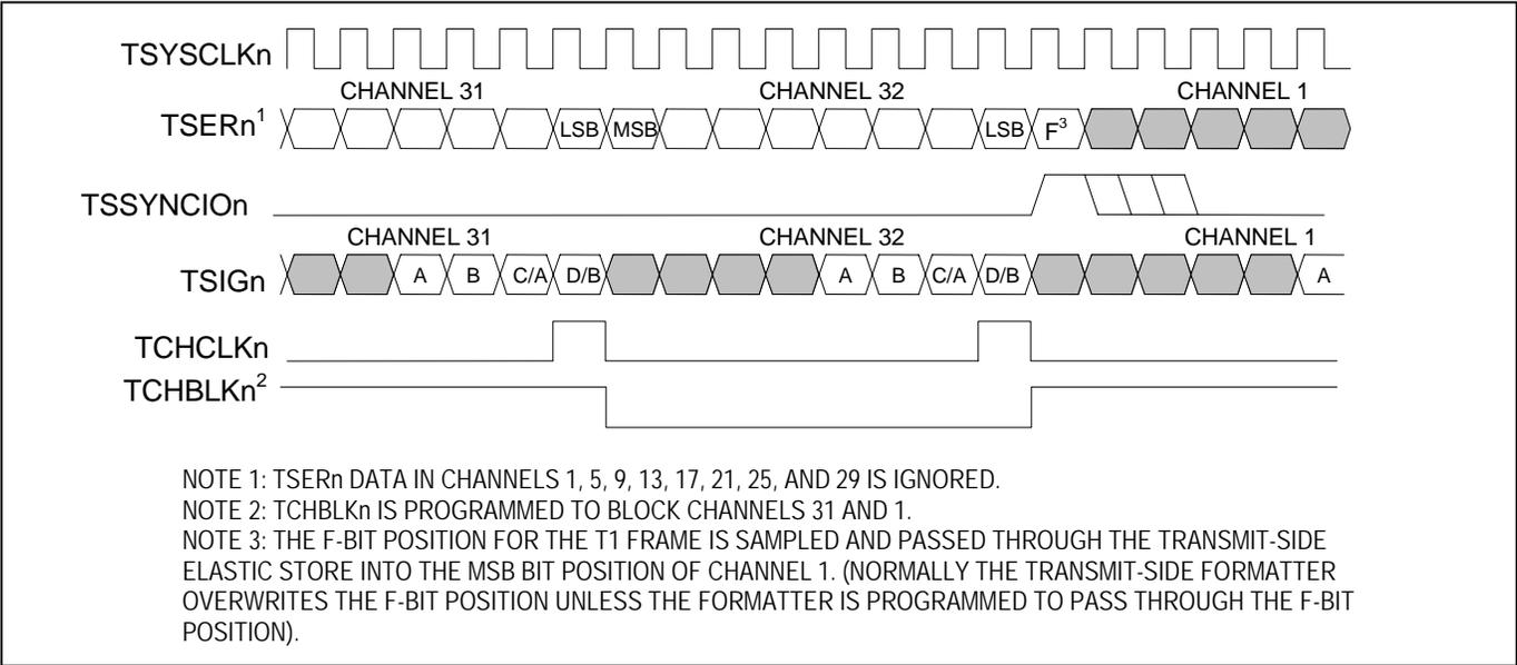
Figure 11-14. T1 Transmit-Side Interleave Bus Operation—BYTE Mode
