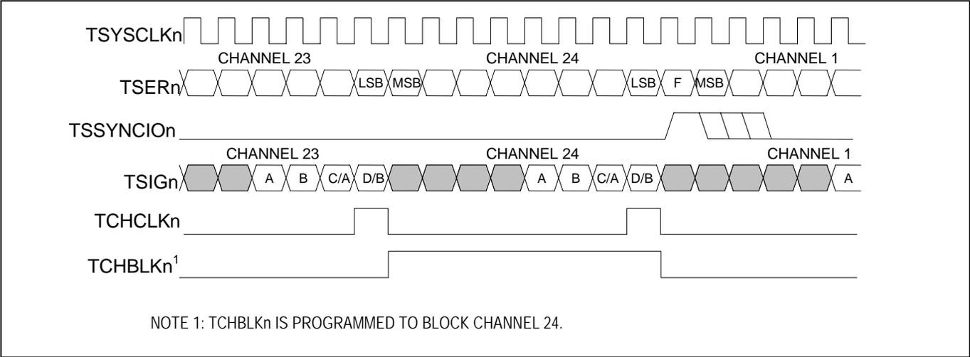
**Figure 11-13. T1 Transmit-Side 2.048MHz Boundary Timing (Elastic Store Enabled)**
