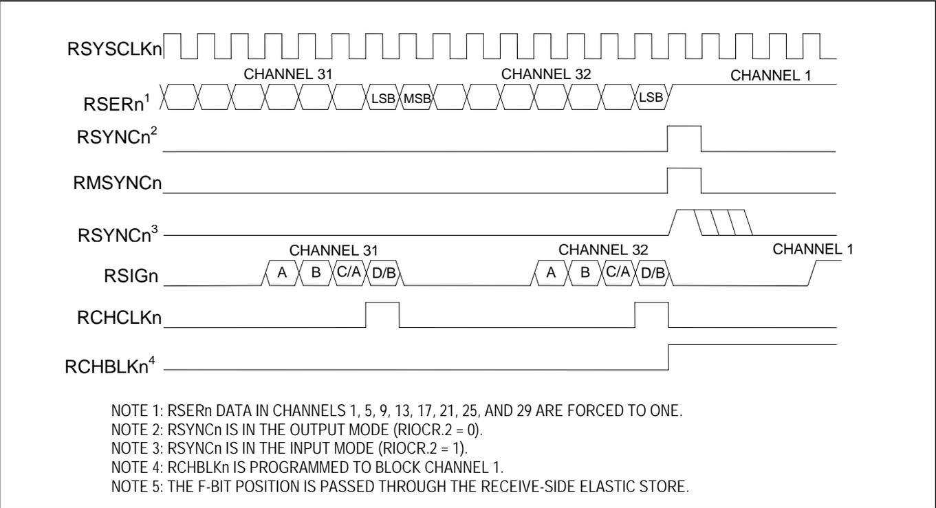
**Figure 11-6. T1 Receive-Side Interleave Bus Operation—BYTE Mode**
