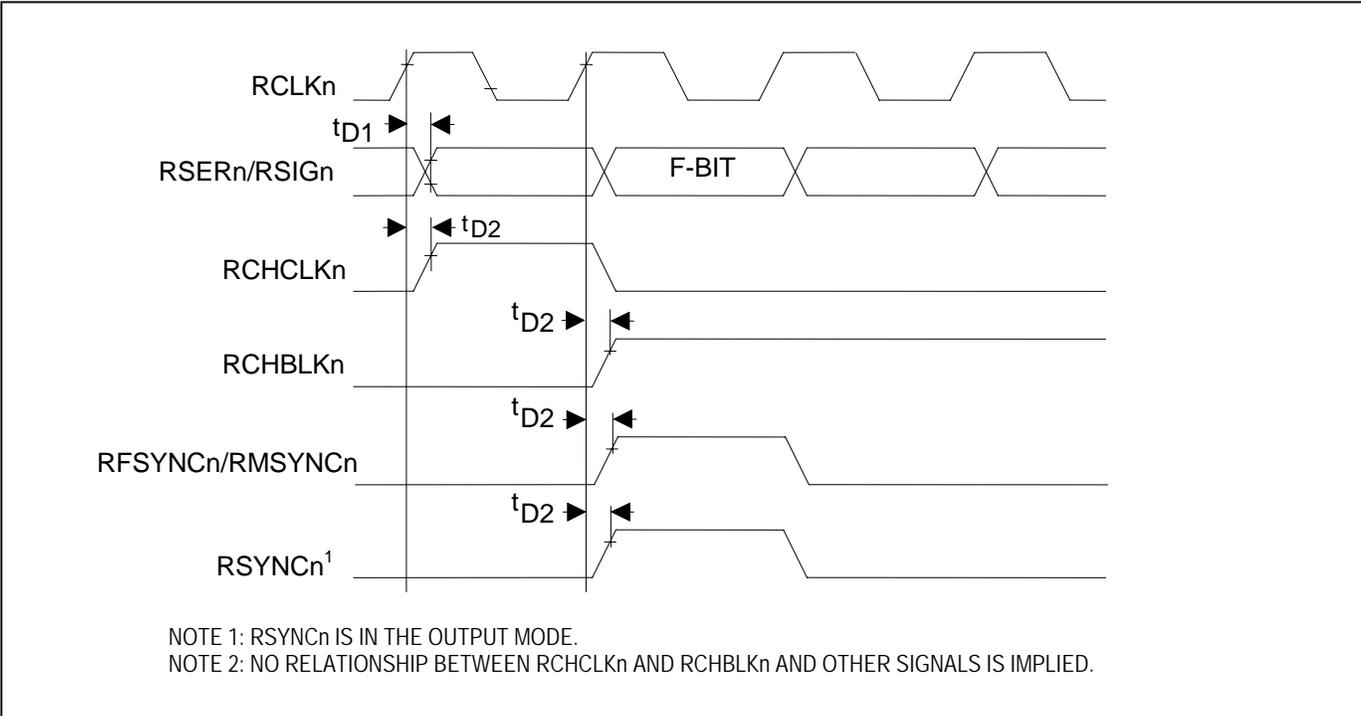
Figure 13-7. Receive-Side Timing—Elastic Store Enabled (T1 Mode)
