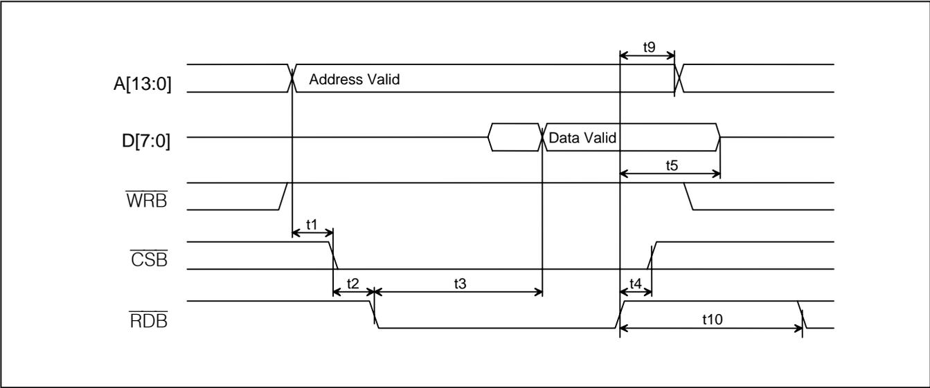
Figure 13-3. Intel Bus Write Timing (BTS = 0)
