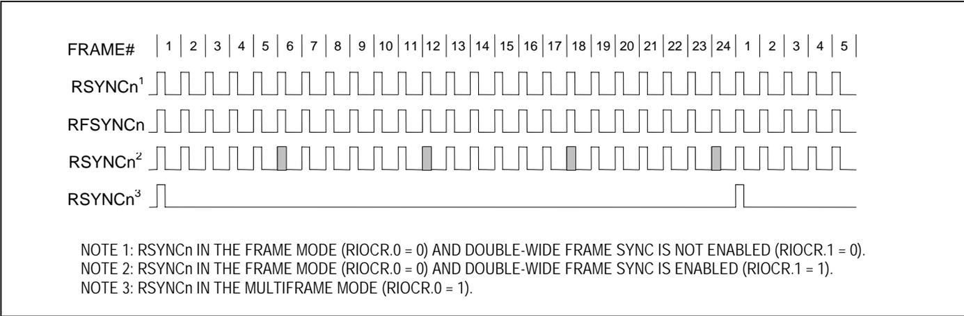
Figure 11-3. T1 Receive-Side Boundary Timing (Elastic Store Disabled)
