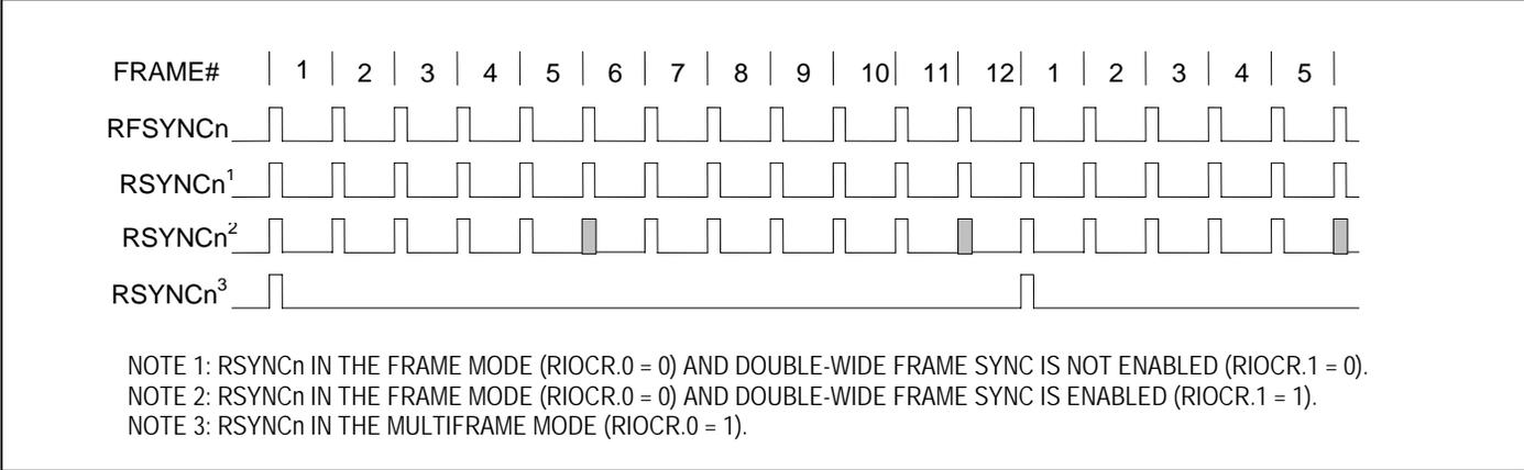
Figure 11-2. T1 Receive-Side ESF Timing
