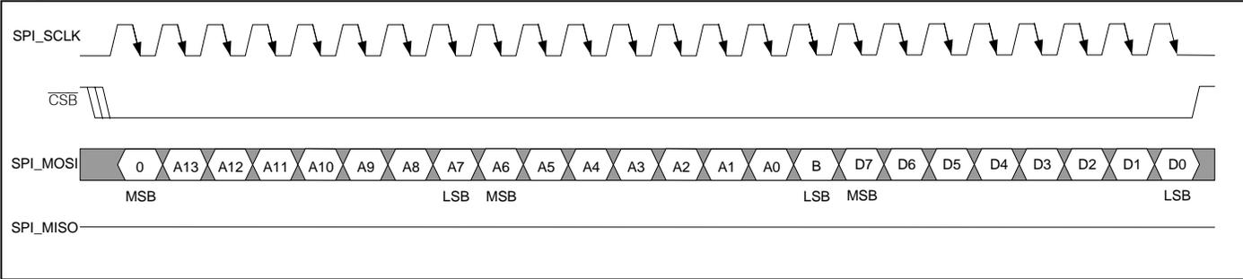
Figure 9-8. SPI Serial Port Access for Write Mode, SPI\_CPOL = 1, SPI\_CPHA = 1
