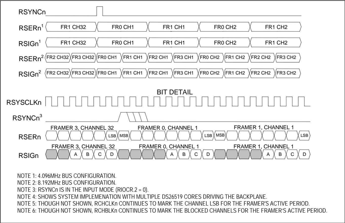
**Figure 11-7. T1 Receive-Side Interleave Bus Operation—FRAME Mode**
