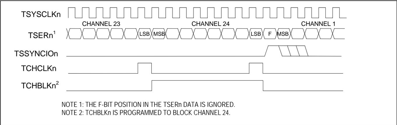
Figure 11-27. E1 Transmit-Side 2.048MHz Boundary Timing (Elastic Store Enabled)
