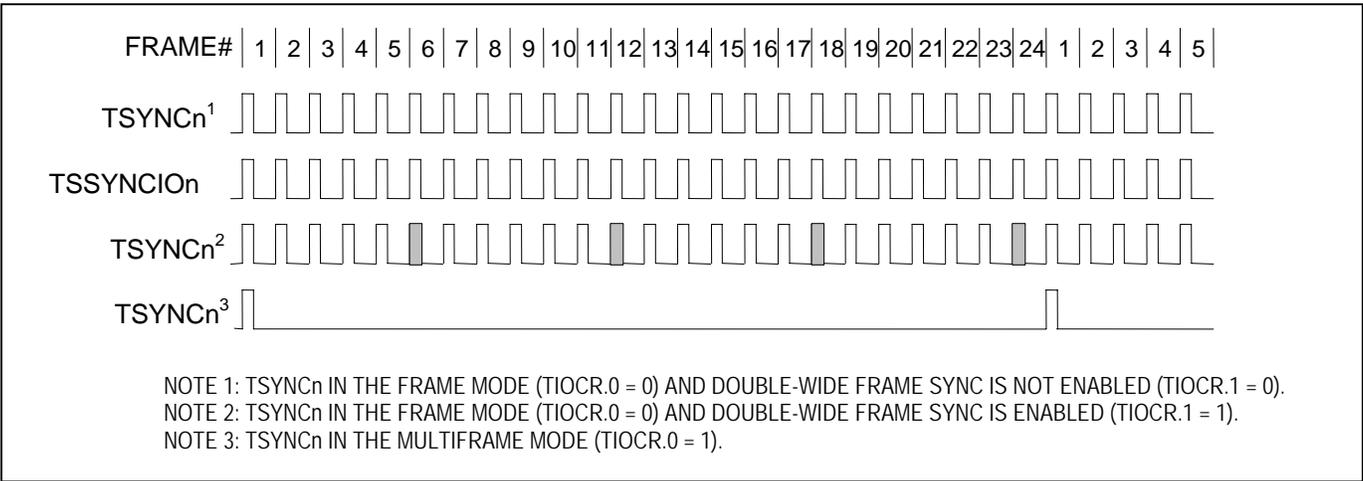
**Figure 11-11. T1 Transmit-Side Boundary Timing (Elastic Store Disabled)**
