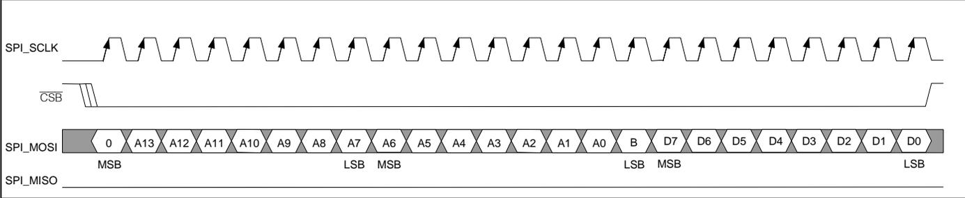
Figure 9-6. SPI Serial Port Access for Write Mode, SPI\_CPOL = 1, SPI\_CPHA = 0
