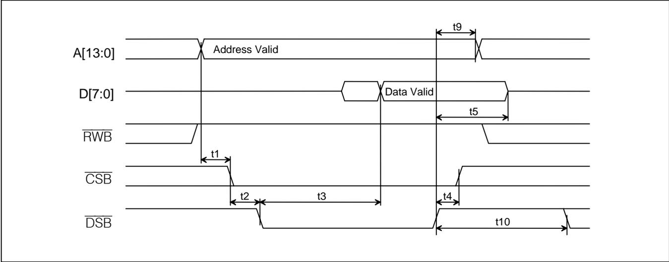
Figure 13-5 Motorola Bus Write Timing (BTS = 1)
