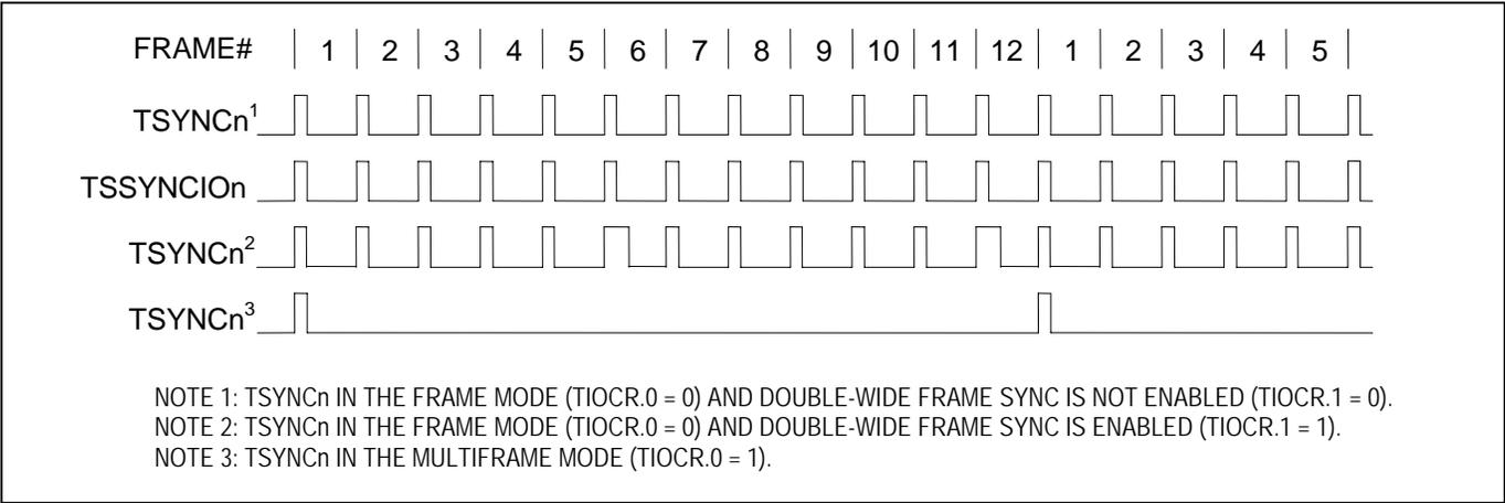
Figure 11-10. T1 Transmit-Side ESF Timing
