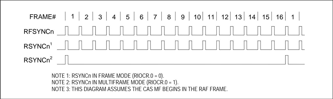
Figure 11-18. E1 Receive-Side Boundary Timing (Elastic Store Disabled)
