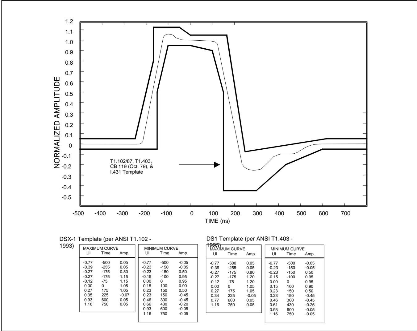
Figure 9-22. E1 Transmit Pulse Templates
