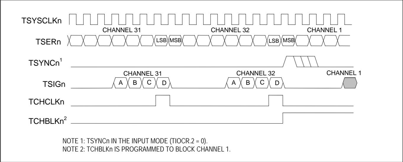
**Figure 11-28. E1 Transmit-Side Interleave Bus Operation—BYTE Mode**
