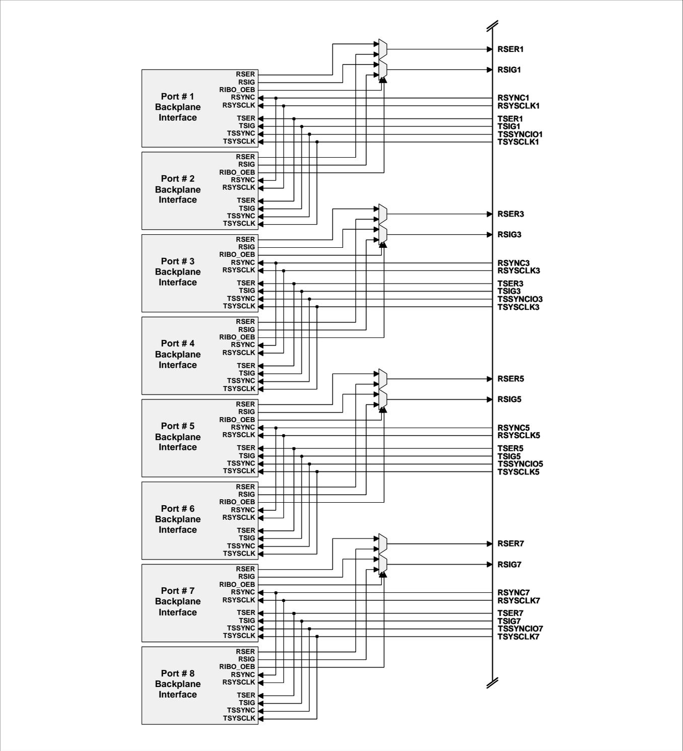
Figure 9-13. IBO Multiplexer Equivalent Circuit—8.192MHz
