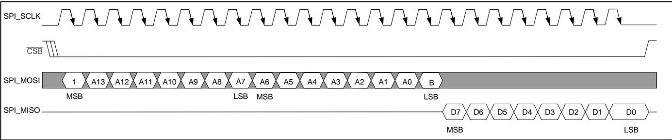
**Figure 9-4. SPI Serial Port Access for Read Mode, SPI\_CPOL = 1, SPI\_CPHA = 1**
