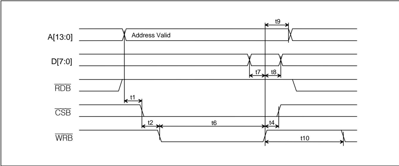
Figure 13-4. Motorola Bus Read Timing (BTS = 1)
