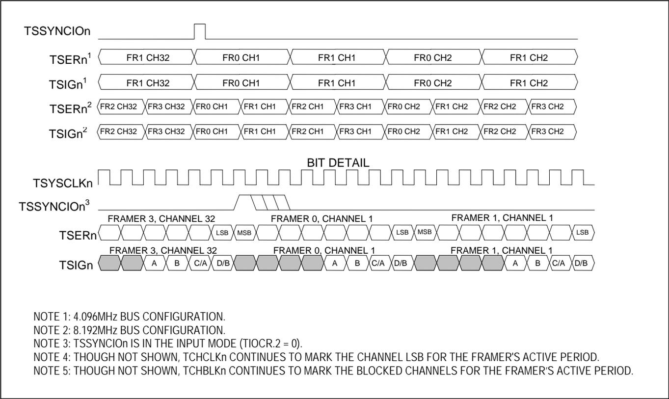
**Figure 11-29. E1 Transmit-Side Interleave Bus Operation—FRAME Mode**
