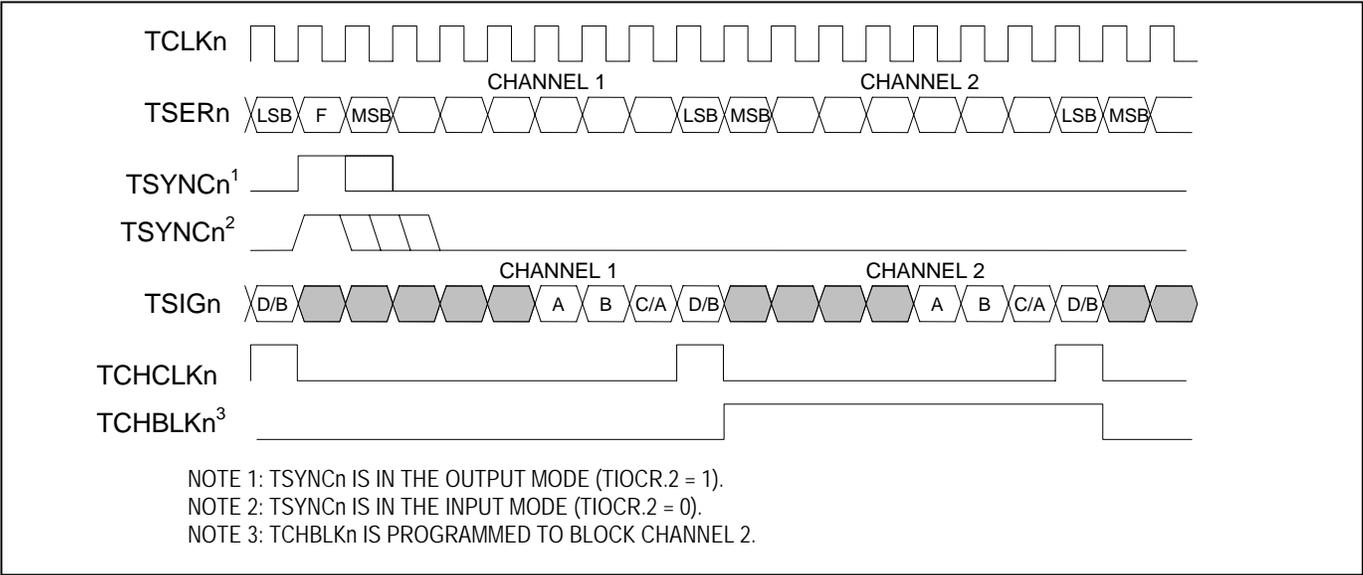
**Figure 11-12. T1 Transmit-Side 1.544MHz Boundary Timing (Elastic Store Enabled)**
