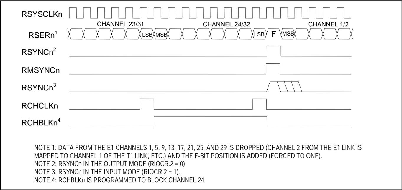
Figure 11-20. E1 Receive-Side 2.048MHz Boundary Timing (Elastic Store Enabled)
