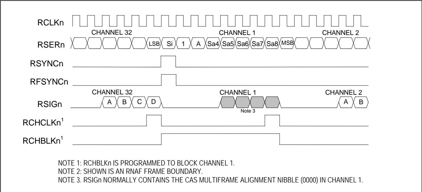
Figure 11-19. E1 Receive-Side 1.544MHz Boundary Timing (Elastic Store Enabled)
