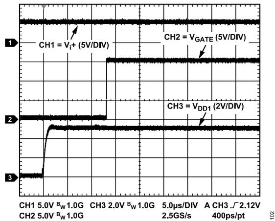
Figure 6. Typical  $V_{DD1}$  Startup to Output Valid
