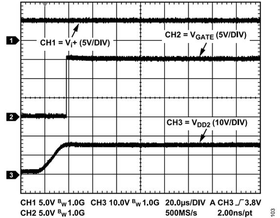
Figure 7. Typical  $V_{DD2}$  Startup to Output Valid
