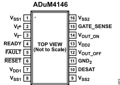
Figure 3. Pin Configuration
