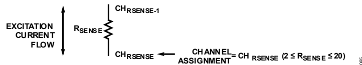
Figure 56. Sense Resistor Channel Assignment Convention for Thermistors
