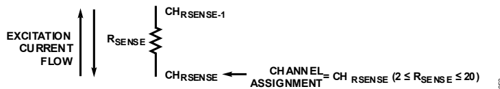
Figure 44. Sense Resistor Channel Assignment Convention for 4-Wire RTDs with Rotation
