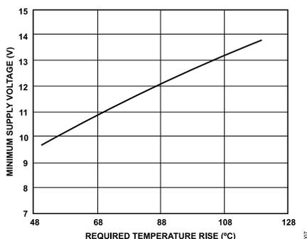
Figure 8. Minimum Supply Voltage vs. Required Temperature Rise
