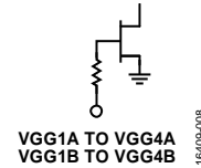
Figure 8. VGG1A to VGG4A and VGG1B to VGG4B Interface Schematic
