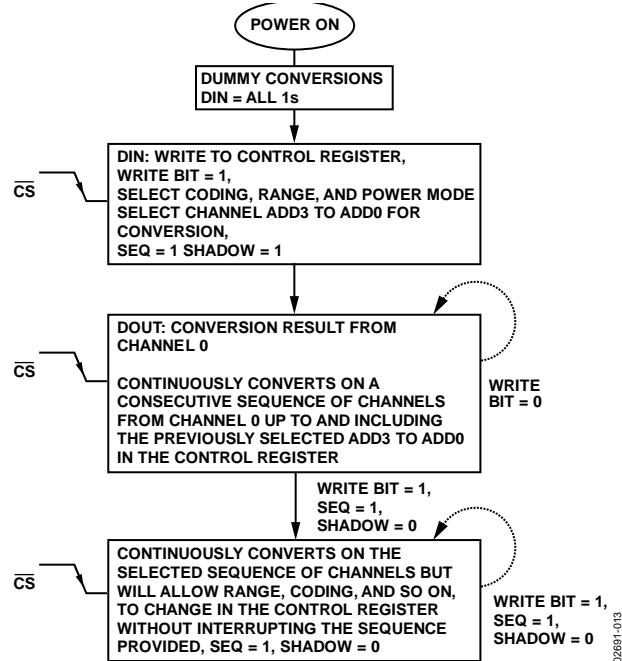
Figure 14. SEQ Bit = 1, SHADOW Bit = 1 Flowchart
