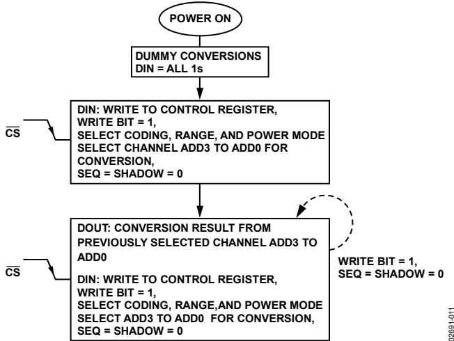
Figure 12. SEQ Bit = 0, SHADOW Bit = 0 Flowchart
