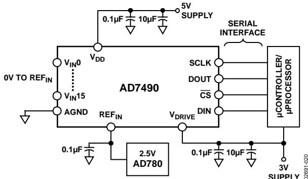
Figure 21. Typical Connection Diagram
