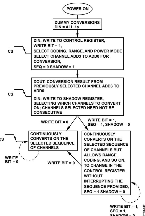
Figure 13. SEQ Bit = 0, SHADOW Bit = 1 Flowchart
