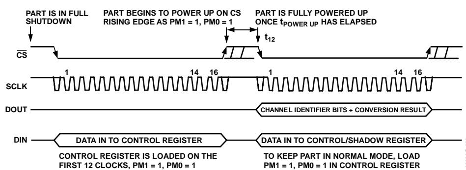
Figure 23. Full Shutdown Mode Operation
