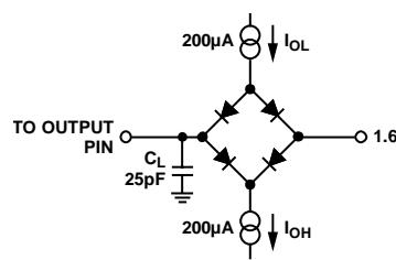
Figure 2. Load Circuit for Digital Output Timing Specifications
