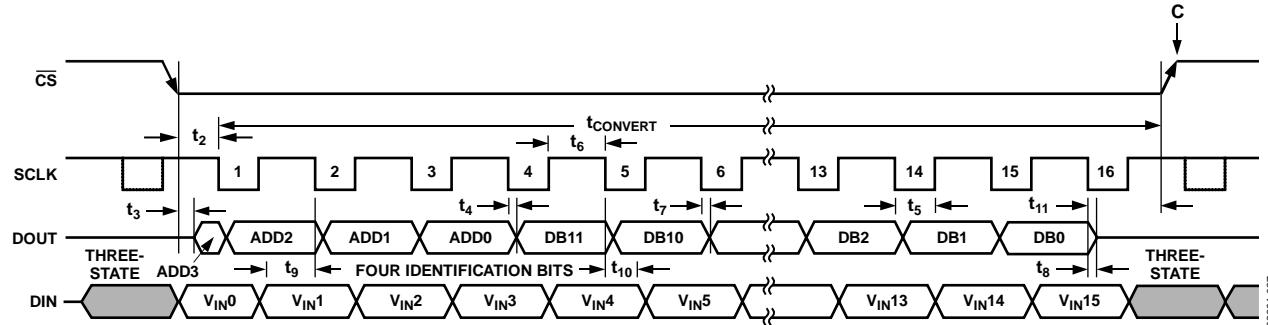
Figure 28. Writing to Shadow Register Timing Diagram
