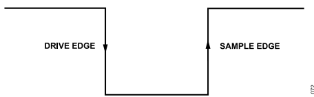
Figure 70. SPI Mode 3, SCLK Edges
