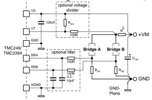
shunt resistor. Place the optional shunt resistor voltage divider near the TMC239, in order to avoid voltage drop in the VCC plane to add up to the measured voltage.
