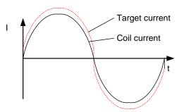
Coil current does not have optimum shape
