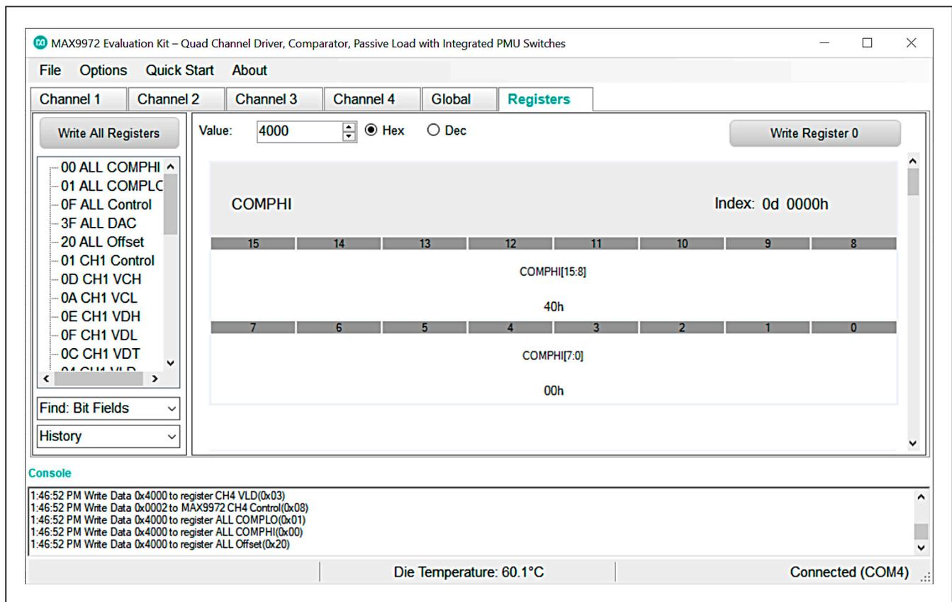
Figure 4. MAX9972 EV Kit Software Window (Register Tab)
