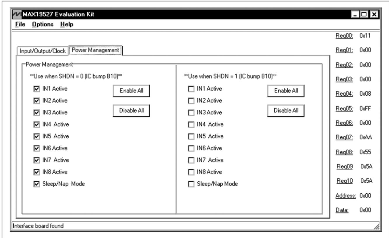
Figure 2. MAX19527 EV Kit Software (Power Management Tab)
