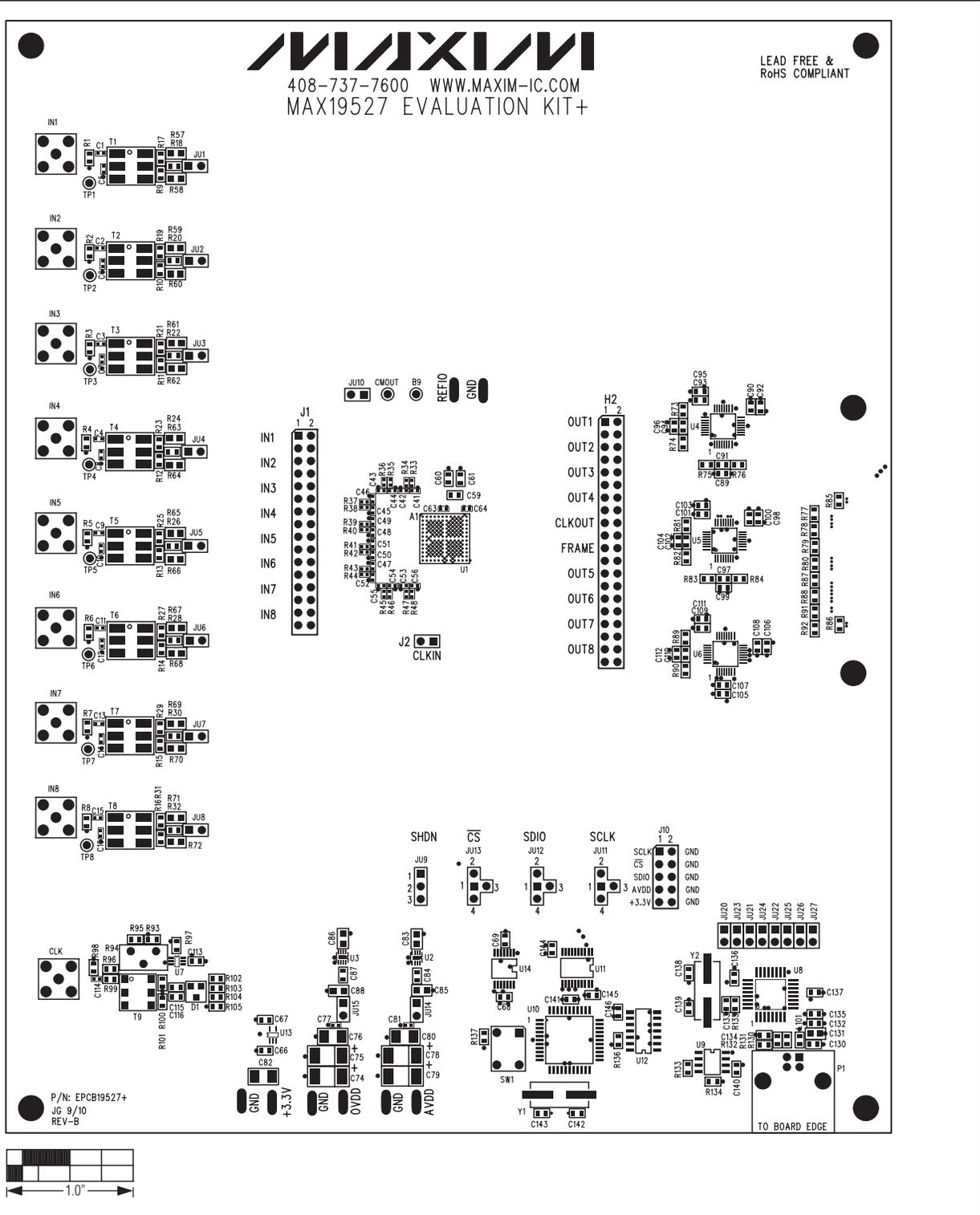
Figure 7. MAX19527 EV Kit Component Placement Guide—Component Side
