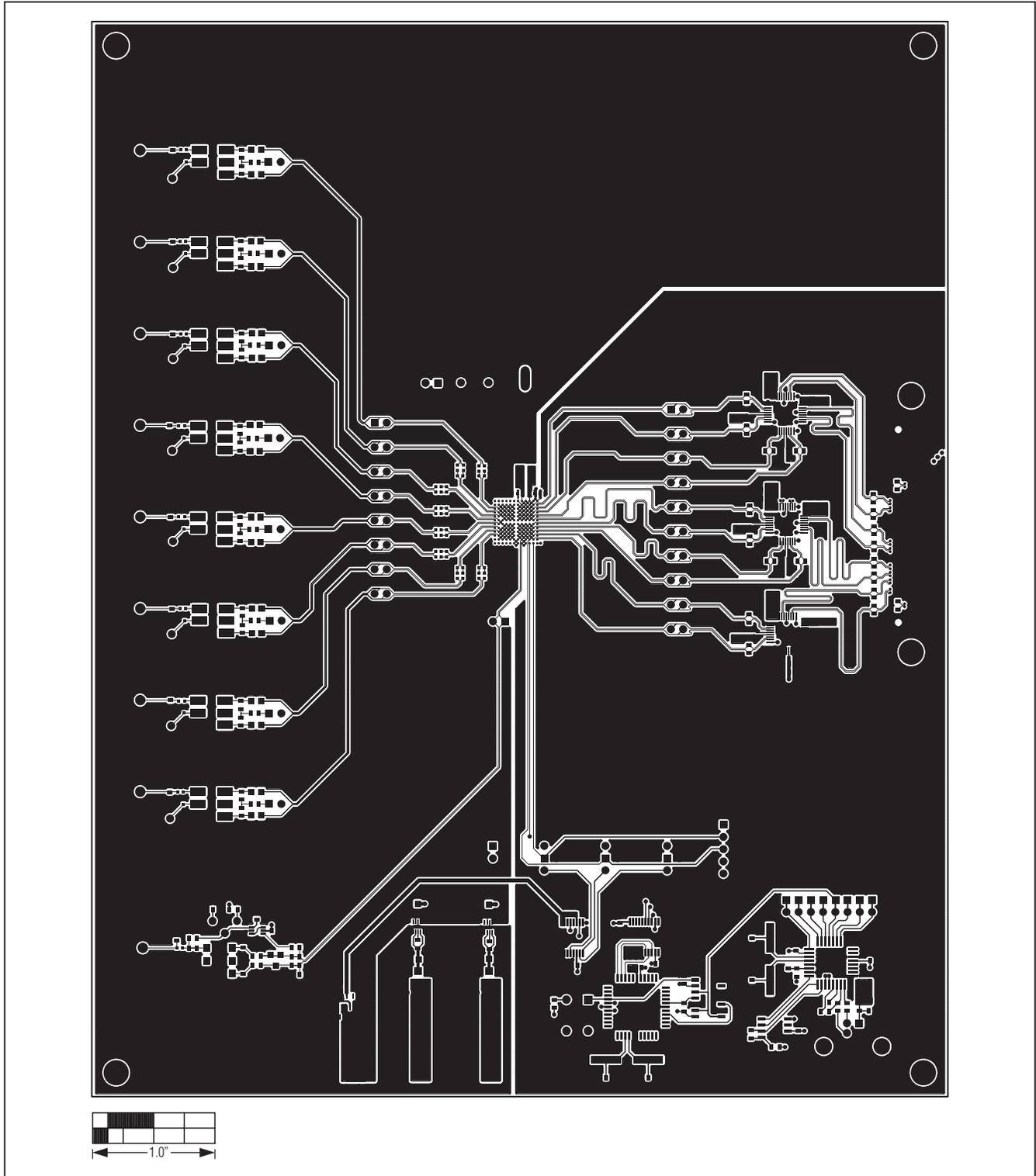
Figure 8. MAX19527 EV Kit PCB Layout—Component Side
