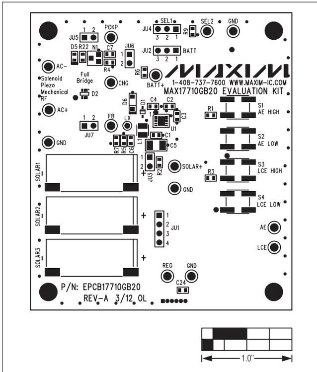
Figure 3. MAX17710GB20 EV Kit Component Placement Guide—Component Side
