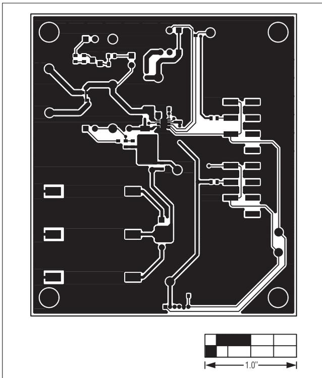
Figure 4. MAX17710GB20 EV Kit PCB Layout—Component Side
