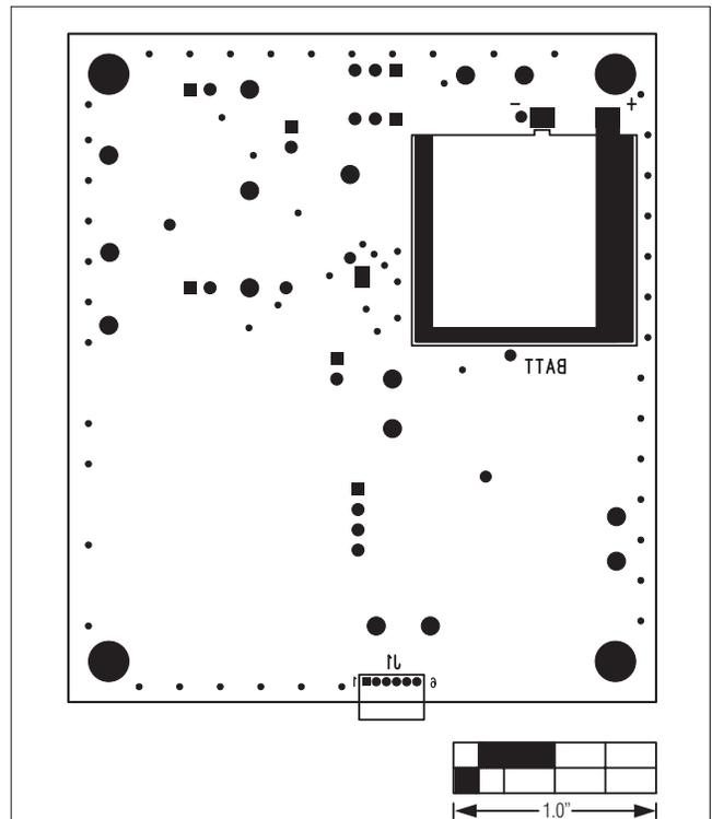
Figure 6. MAX17710GB20 EV Kit Component Placement Guide—Solder Side
