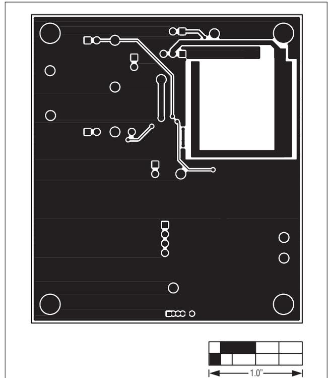
Figure 5. MAX17710GB20 EV Kit PCB Layout—Solder Side
