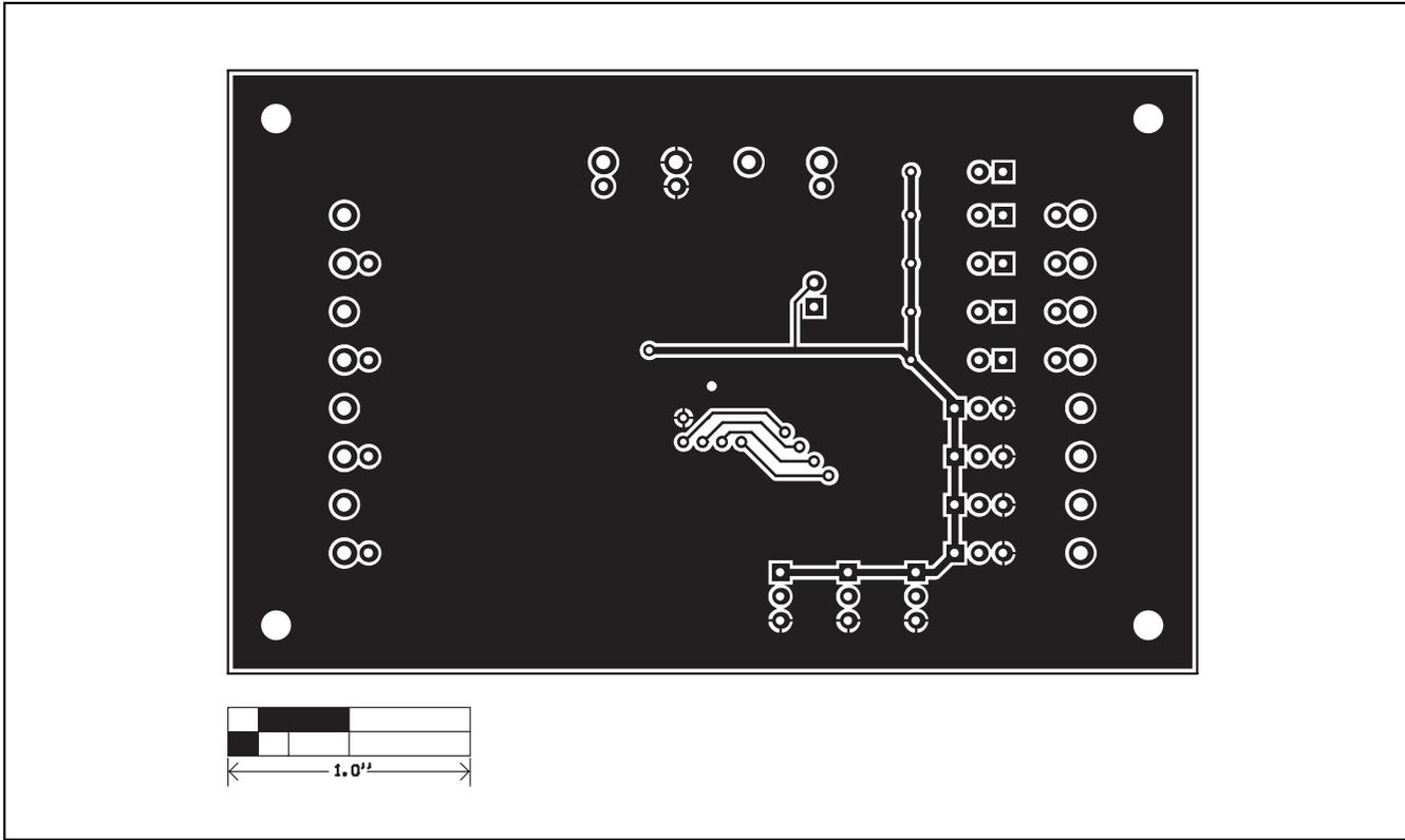
Figure 4. MAX16029EV Kit PCB Layout—Solder Side
