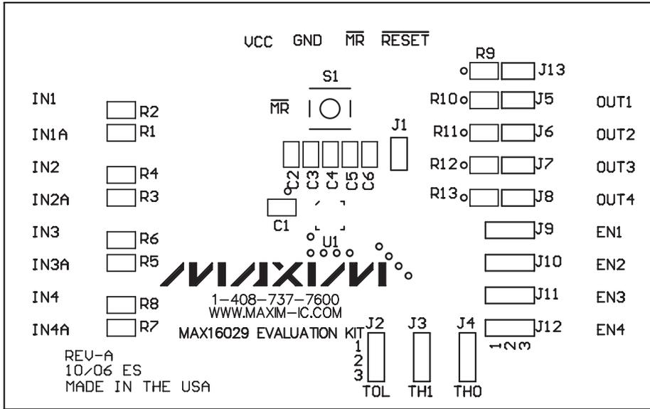
Figure 2. MAX16029EV Kit Component Placement Guide—Components Side
