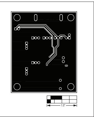
Figure 6. MAX14585 EV Kit PCB Layout—Solder Side
