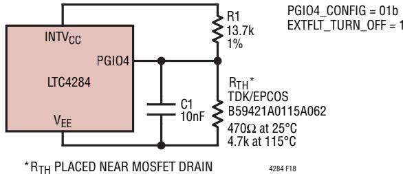
**Figure 18.** Use PGPIO4/EXT\_FAULT to Turn Off MOSFET when Drain Temperature Exceeds 115°C
