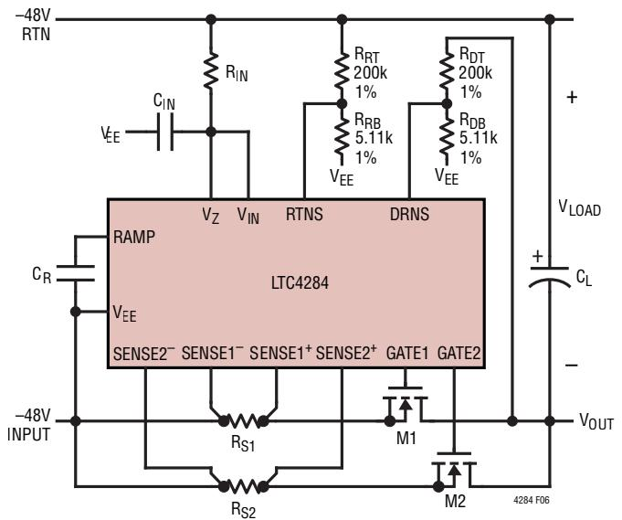
Figure 6. dV/dt Inrush Control Using RAMP Capacitor
