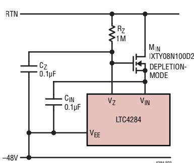
Figure 3. The LTC4284 Can Operate to &gt;300V Using a Depletion Mode N-Channel MOSFET
