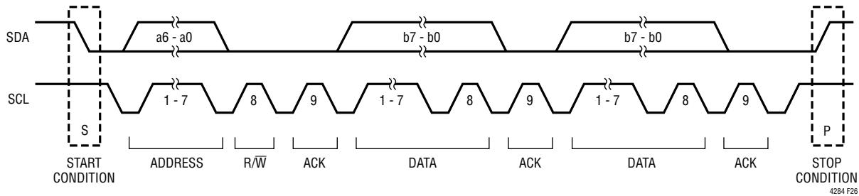
Figure 26. General Data Transfer over I<sup>2</sup>C
