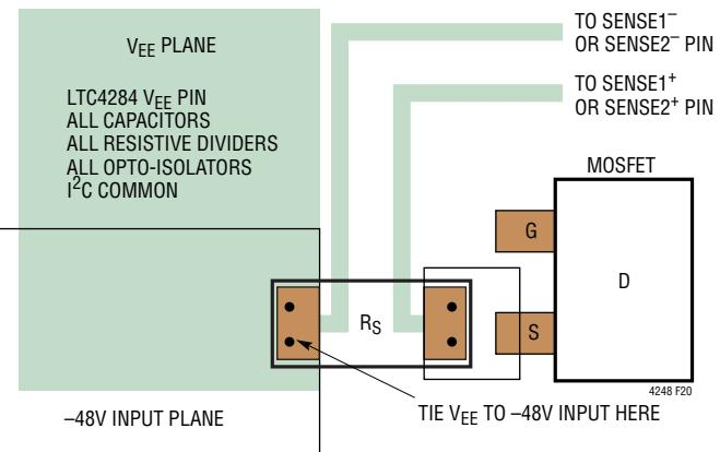
Figure 20. Layout Example of V<sub>EE</sub> Plane, –48V Input Plane and Sense Resistor Connection
