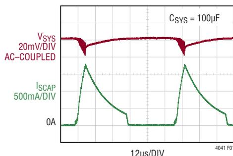
Figure 1. Charge Current Waveform for  $V_{SCAP} < 1V$
