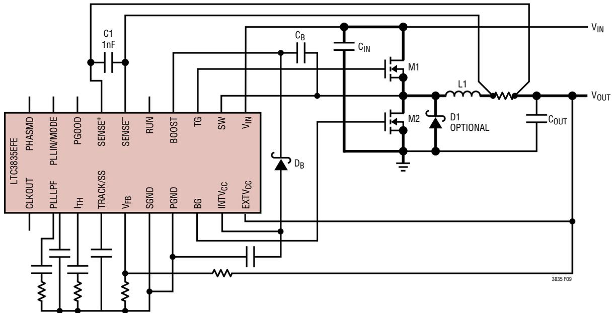
Figure 9. LTC3835 Recommended Printed Circuit Layout Diagram
