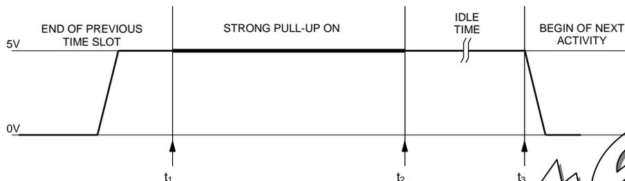
The minimum duration of a strong pull-up of infinite duration strongly depends on the baud rate of the communication between host and DS2480. The host must first receive the response byte of the single-bit command, react to it and then transmit the termination command. Neglecting the host's response time, the shortest duration of an infinite strong pull-up therefore is 173.6  $\mu$ s at 115.2 kbps, 347.2  $\mu$ s at 57.6 kbps, 1.04 ms at 19.2 kbps and 2.08 ms at 9.6 kbps.
