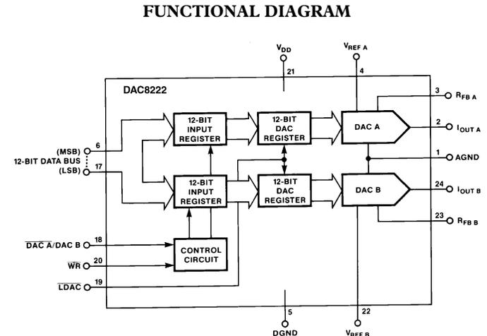
double-buffered digital inputs will allow both DACs to be simultaneously updated.
