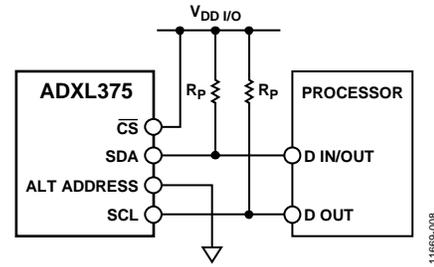
Figure 28. I<sup>2</sup>C Connection Diagram (Address 0x53)
