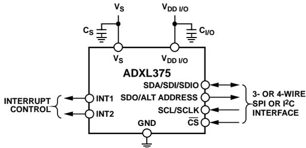
Figure 31. Application Diagram
