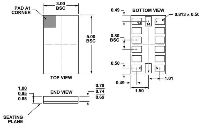
Figure 40. 14-Terminal Land Grid Array [LGA] (CC-14-1)
