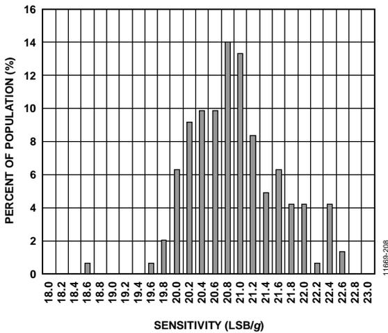
Figure 12. Z-Axis Sensitivity at 25°C,  $V_S = 2.5 V$
