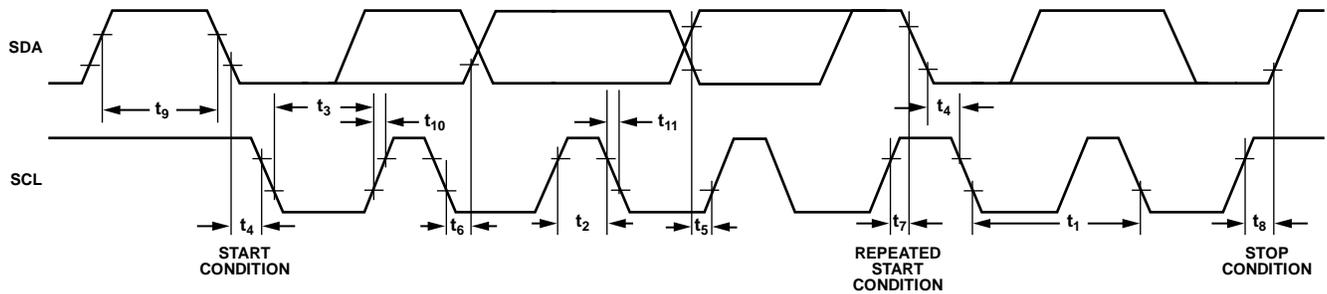
Figure 30. I<sup>2</sup>C Timing Diagram
