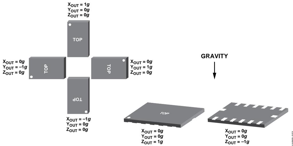
Figure 37. Output Response vs. Orientation to Gravity
