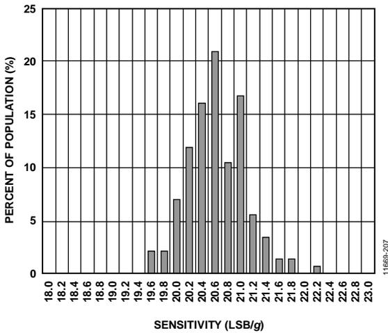
Figure 11. Y-Axis Sensitivity at 25°C,  $V_S = 2.5 V$
