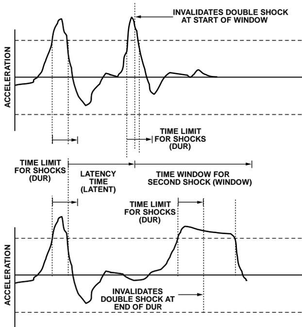
Figure 35. Shock Interrupt Function with Invalid Double Shocks
