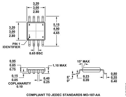
**Figure 42. 8-Lead Mini Small Outline Package [MSOP]
