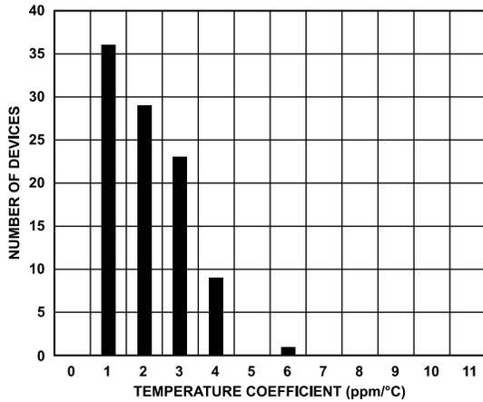
Figure 4. ADR3525 Temperature Coefficient Distribution
