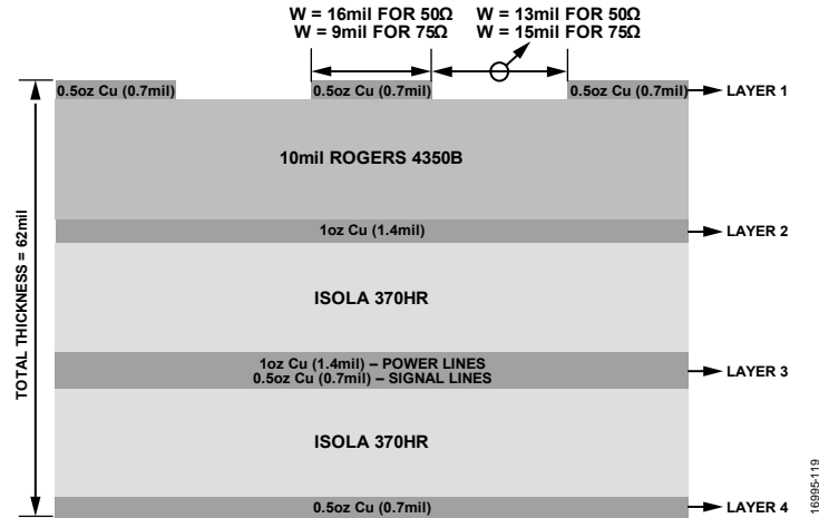
Figure 127. ADMV4420-EVALZ PCB, Cross Sectional View
