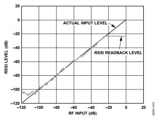
Figure 15. Digital RSSI Readback Linearity
