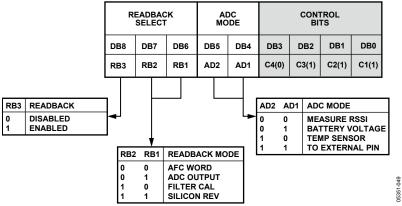
Figure 52. Register 7—Readback Setup Register
