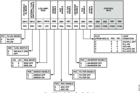
Figure 53. Register 8—Power-Down Test Register
