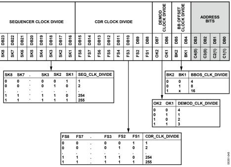
Figure 48. Register 3—Receiver Clock Register
