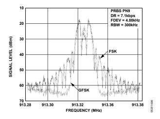
Figure 8. Output Spectrum in FSK and GFSK Modulation
