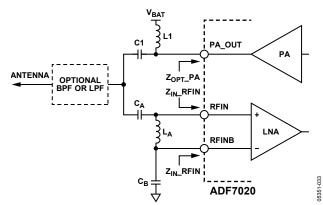
Figure 33. ADF7020 with Internal Rx/Tx Switch
