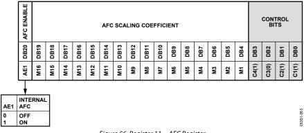
Figure 56. Register 11—AFC Register
