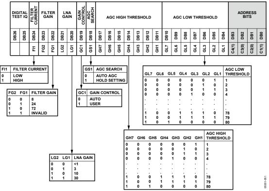
Figure 54. Register 9—AGC Register
