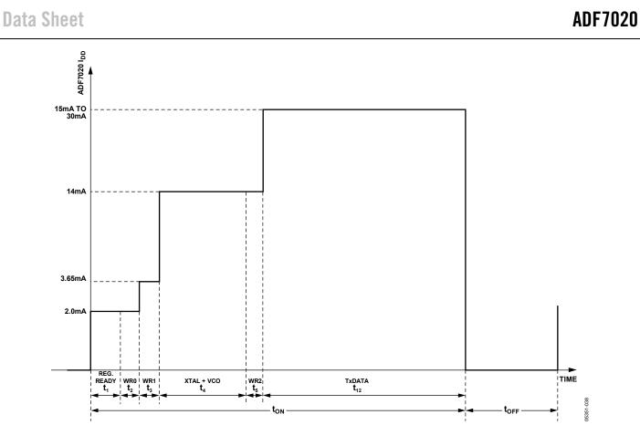
Figure 40. Tx Programming Sequence and Timing Diagram
