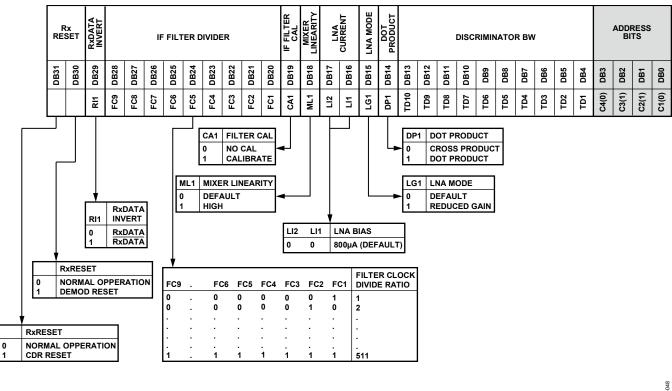
Figure 51. Register 6—Correlator/Demodulator Register
