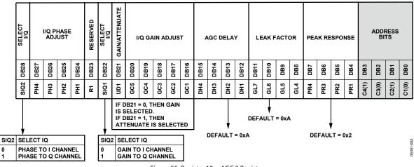
Figure 55. Register 10—AGC 2 Register
