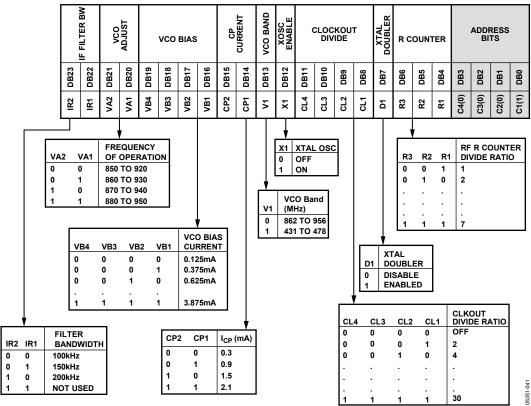
*Figure 44. Register 1—Oscillator/Filter Register*
