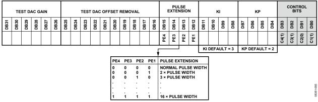
Figure 58. Register 13—Offset Removal and Signal Gain Register
