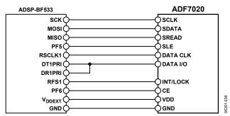
Figure 38. ADSP-BF533 to ADF7020 Connection Diagram
