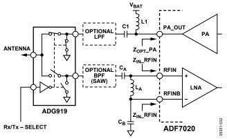
Figure 32. ADF7020 with External Rx/Tx Switch
