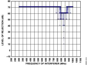
Figure 14. Wideband Interference Rejection; Wanted Signal (880 MHz) at 3 dB above Sensitivity Point Interferer = FM Jammer (9.76 kbps, 10 kHz Deviation)
