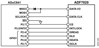
Figure 37. ADuC841 to ADF7020 Connection Diagram
