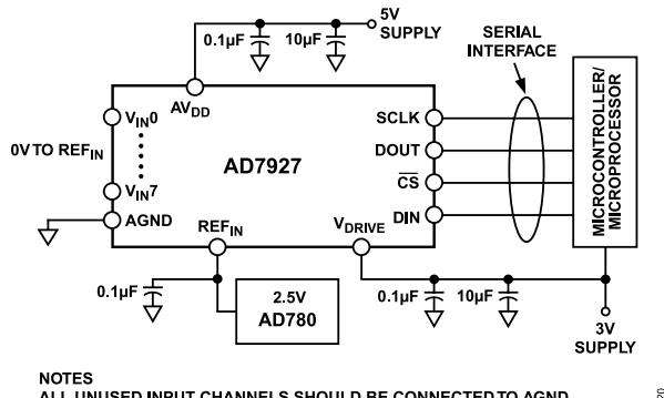
Figure 20. Typical Connection Diagram
