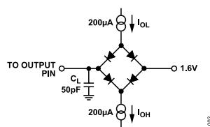
**Figure 2. Load Circuit for Digital Output Timing Specifications**
