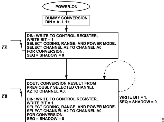
Figure 11. SEQ Bit = 0, SHADOW Bit = 0 Flowchart
