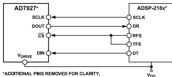
Figure 30. Interfacing to the ADSP-218x
