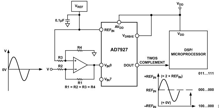
Figure 19. Handling Bipolar Signals
