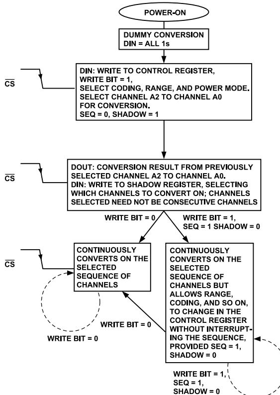
Figure 12. SEQ and SHADOW Conversion Flowchart to Continuously Convert a Sequence of Channels
