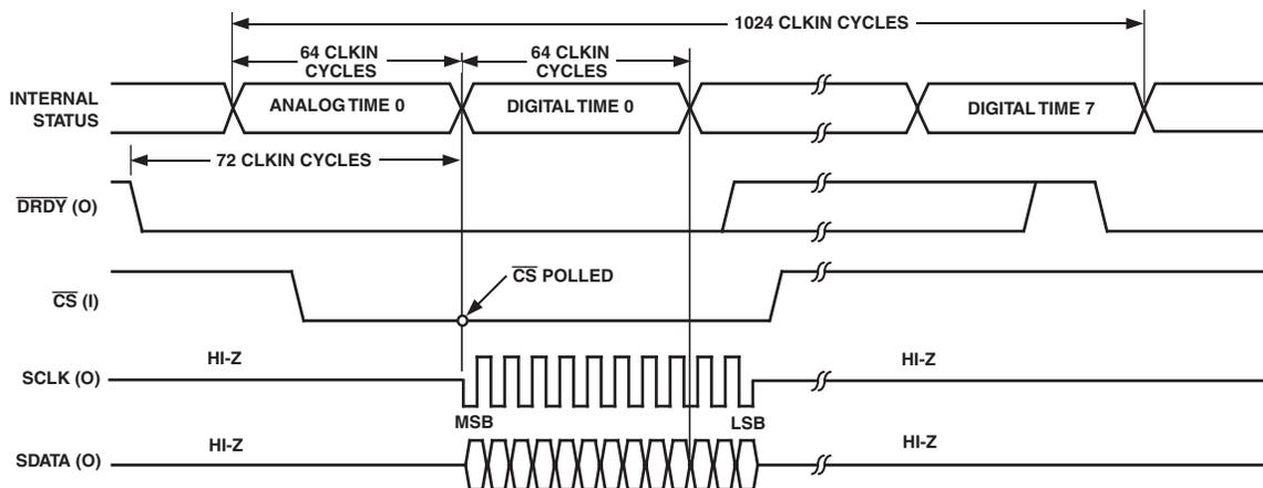
Figure 15. Timing Diagram for SSC Transmission Mode
