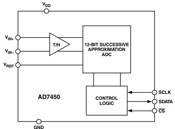
The AD7450 uses advanced design techniques to achieve low power dissipation at high throughput rates.
