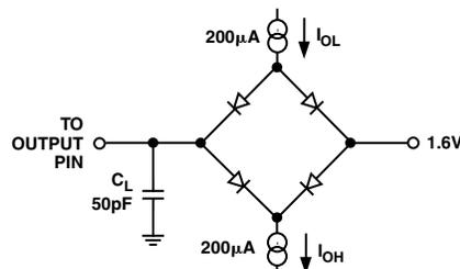
Figure 2. Load Circuit for Digital Output Timing Specifications
