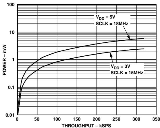
Figure 24. Power vs. Throughput Rate for Power-Down Mode
