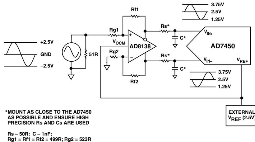
Figure 14. Using the AD8138 as a Single-Ended-to-Differential Amplifier
