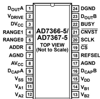
Figure 2. Pin Configuration
