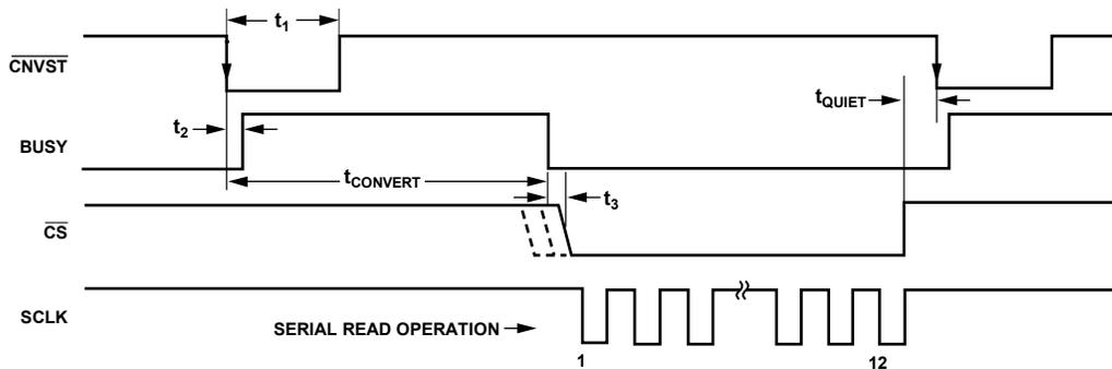
Figure 22. Normal Mode Operation for the AD7366-5
