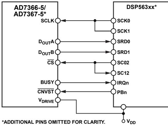
Figure 32. Interfacing the AD7366-5/AD7367-5 to the DSP563xx
