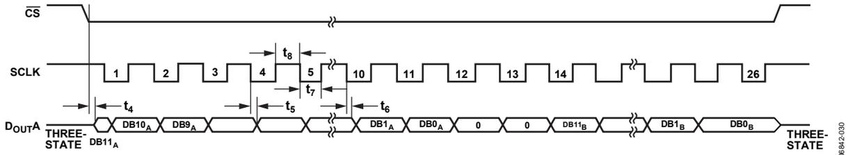
Figure 27. Reading Data from Both ADCs on One D<sub>OUT</sub> Line with 24 SCLKs for the AD7366-5
