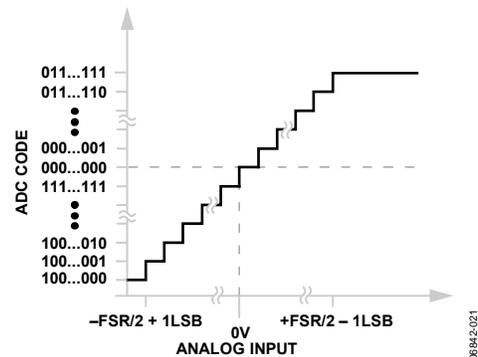
Figure 19. Transfer Characteristic
