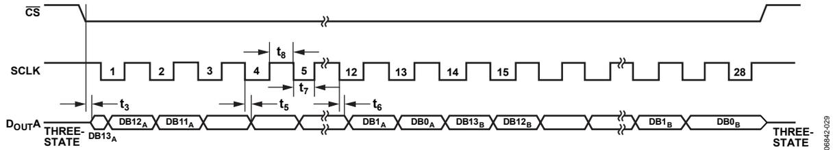
Figure 28. Reading Data from Both ADCs on One D<sub>OUT</sub> Line with 28 SCLKs for the AD7367-5
