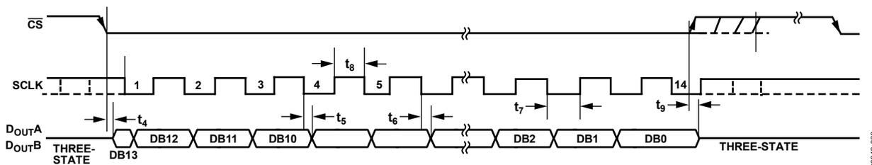
Figure 26. Serial Interface Timing Diagram for the AD7367-5
