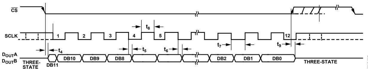
Figure 25. Serial Interface Timing Diagram for the AD7366-5
