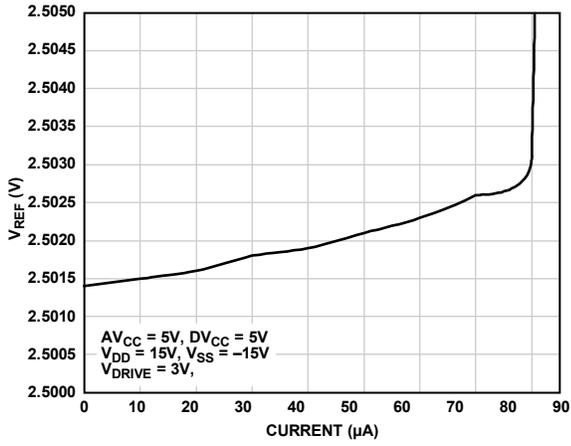
Figure 13.  $V_{REF}$  vs. Reference Output Current Drive
