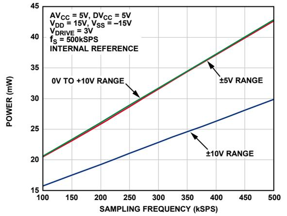
Figure 15. Power vs. Sampling Frequency in Normal Mode
