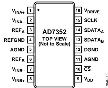
Figure 2. Pin Configuration
