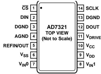
Figure 3. Pin Configuration
