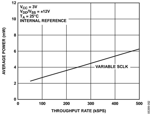
Figure 48. Power vs. Throughput Rate with 3 V  $V_{CC}$
