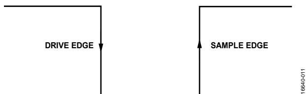
Figure 32. SPI Mode 3 SCLK Edges
