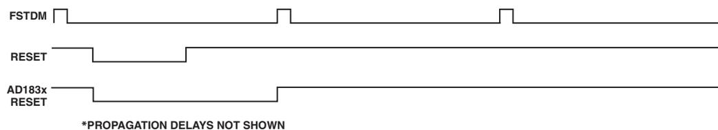
Figure 4. Reset Synchronized to Rising Edge of FSTDM/ALRCLK
