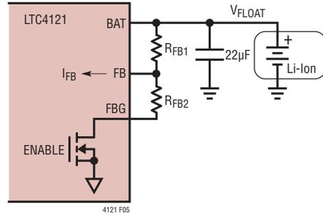
Figure 5. Programming the Float Voltage with LTC4121
