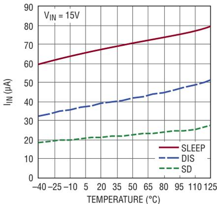
BAT Pin Sleep/Shutdown Current vs Temperature
