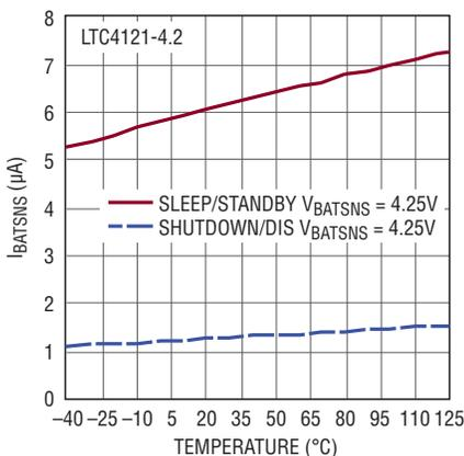
BAT Pin Standby/Sleep/Shutdown Current vs Temperature
