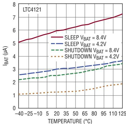
Feedback Pin Standby or Sleep/Disabled Current vs Temperature
