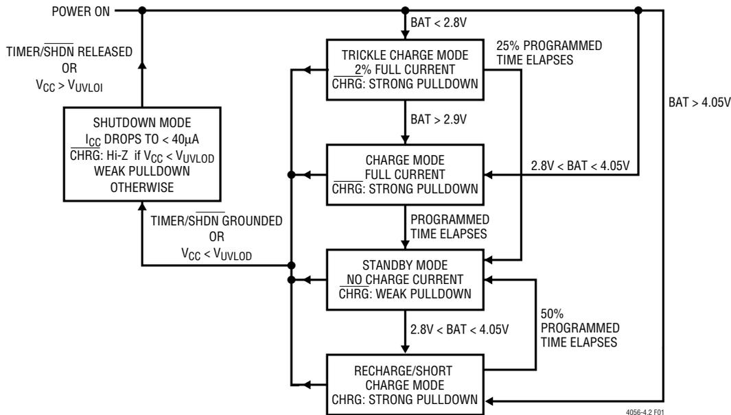
Figure 1. State Diagram for a Typical Charge Cycle
