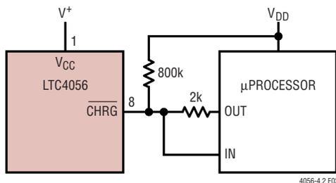
Figure 2. Using a Microprocessor to Determine  $\overline{\text{CHRG}}$  State
