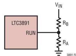
Figure 4. Using the RUN Pin as a UVLO
