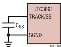
Figure 5. Using the TRACK/SS Pin to Program Soft-Start
