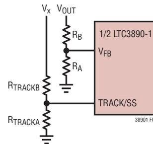
**Figure 8. Using the TRACK/SS Pin for Tracking**
