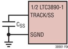
**Figure 6. Using the TRACK/SS Pin to Program Soft-Start**
