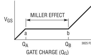
Figure 6. Gate Charge Curve
